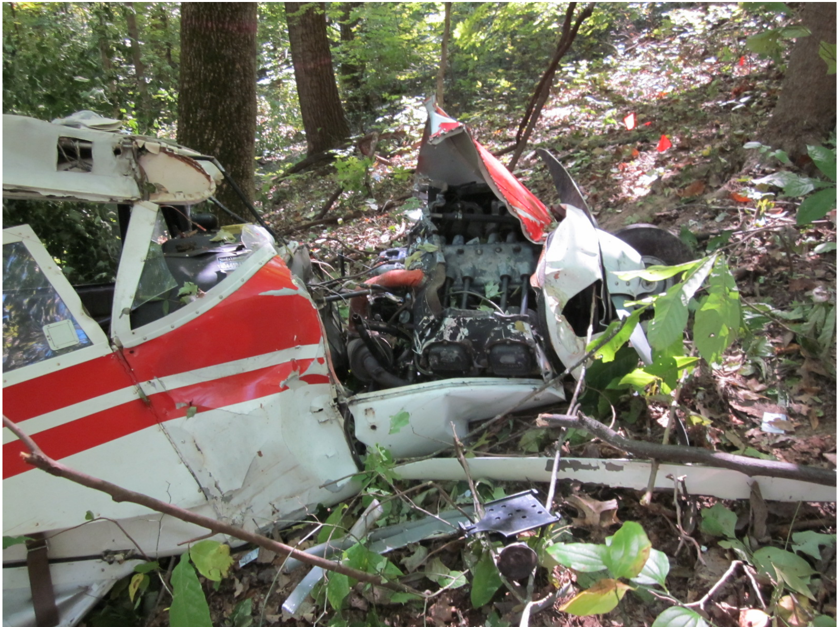
Photo 4 – View of Engine Separated from the Firewall (Photo Courtesy of FAA)
