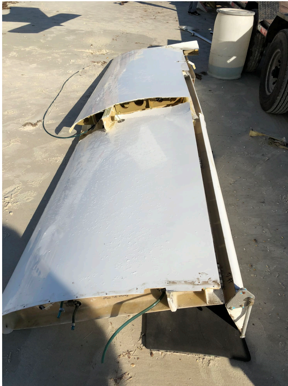
Photo 2 – View of broken right wing and spar. (Courtesy of FAA)
