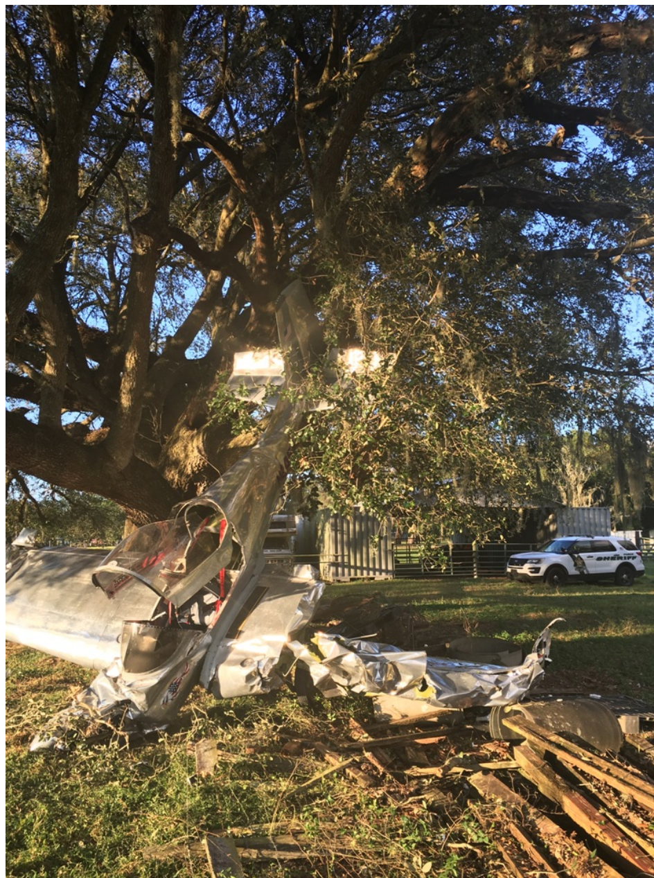
Photo 2 - FAA Digital Photograph. Left Forward Quartering View Depicting Wreckage at Accident Site. Note the extensively damaged left wing.
