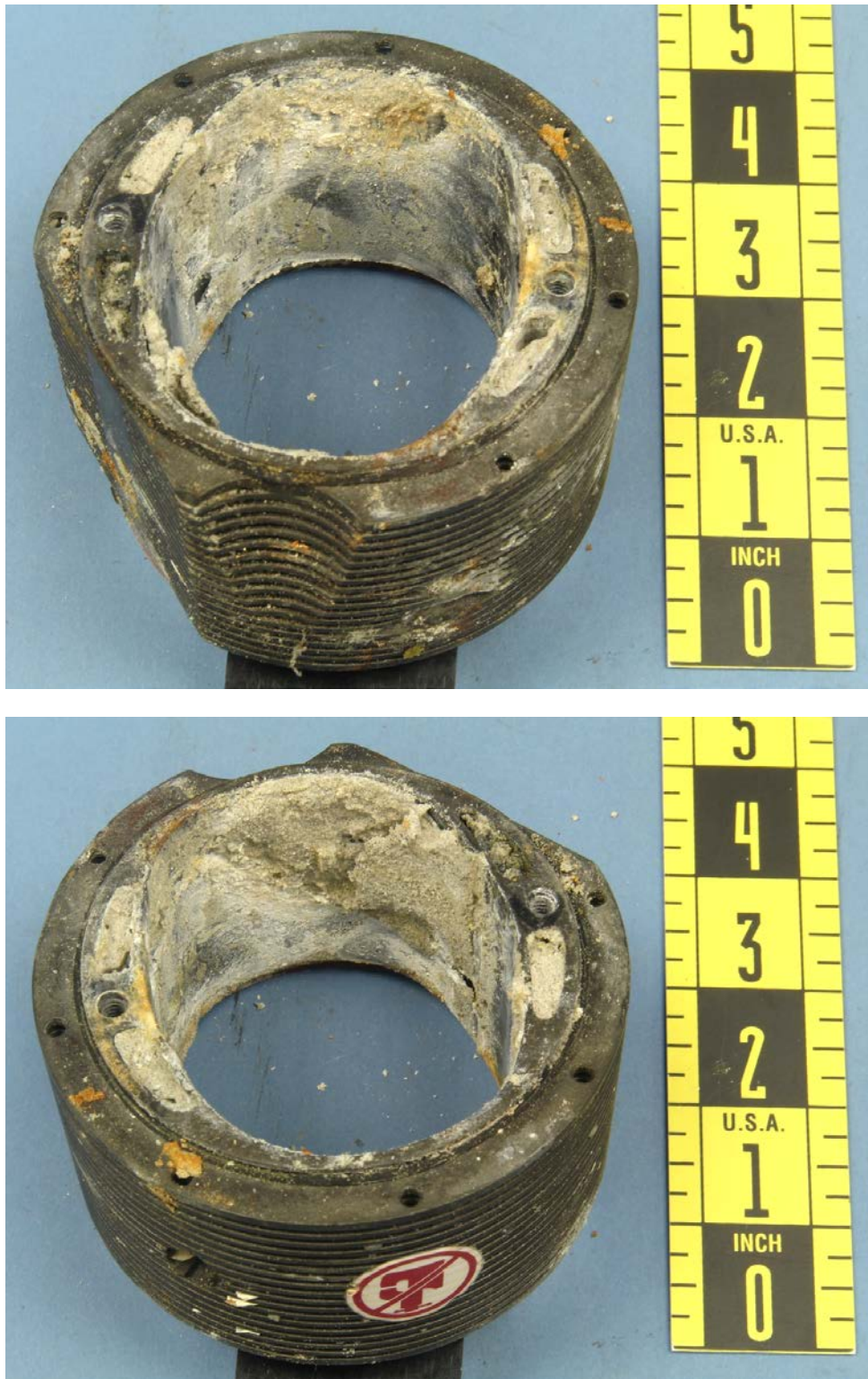
Figure 2: Overall photos showing the corrosion deposits on the inner diameter surface of the vacuum pump housing.
