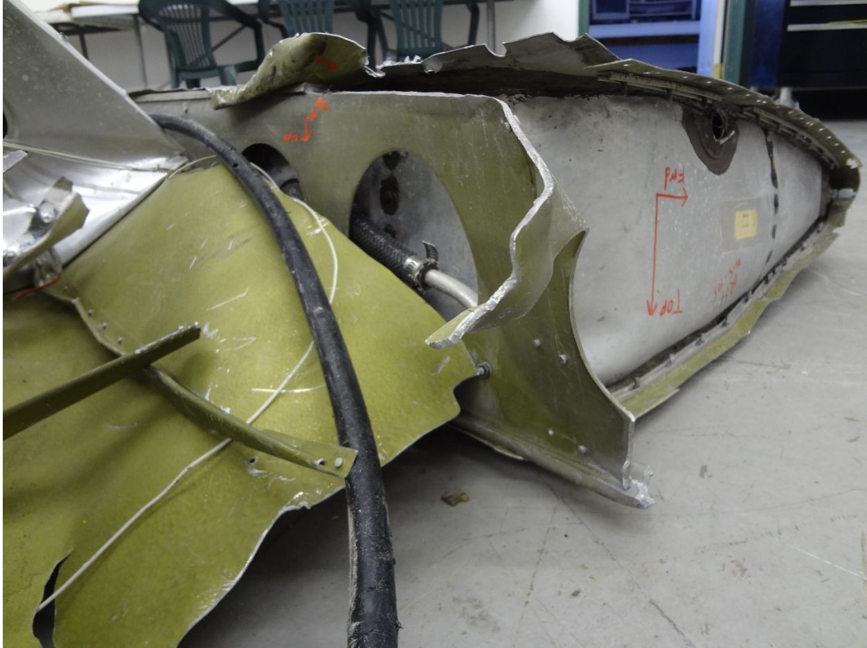
Figure 5: Right Wing Fracture Surface (Photo Courtesy of Piper Aircraft)
