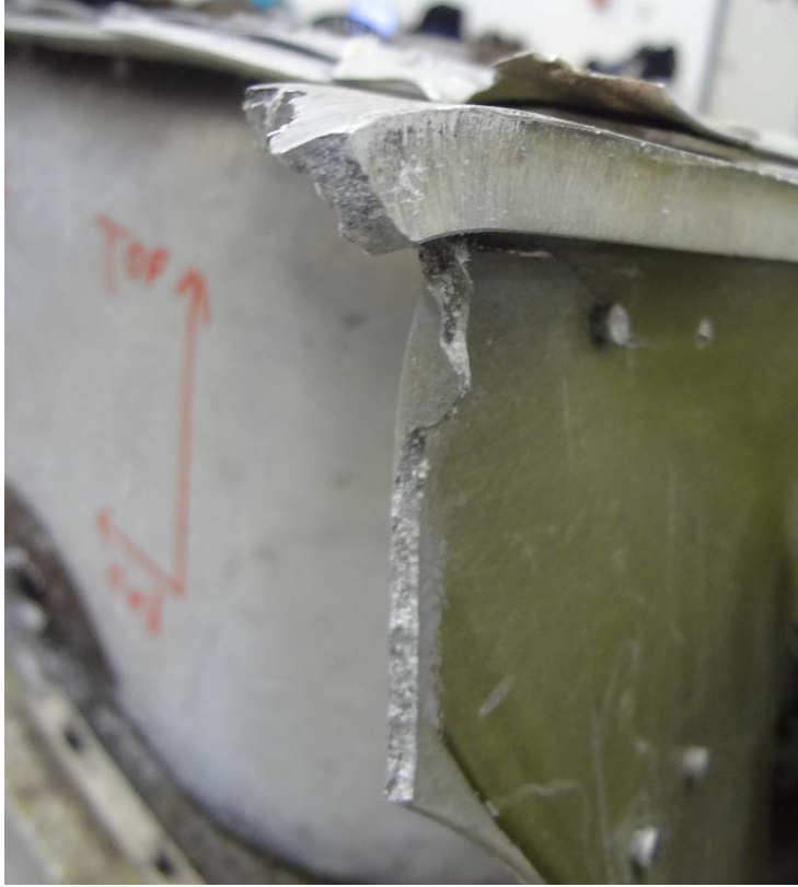
Figure 7: Right Wing Upper Fracture Surface (Photo Courtesy of Piper Aircraft)
