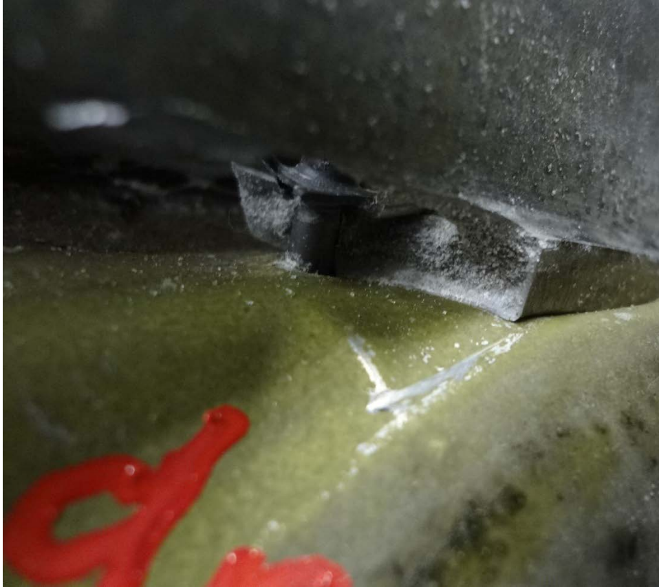
Figure 8: Right Wing Lower Fracture Surface (Photo Courtesy of Piper Aircraft)
