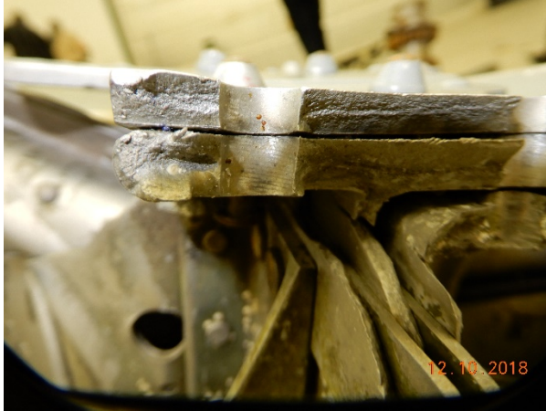
Figure 14: Left Wing Lower Fracture Surface
