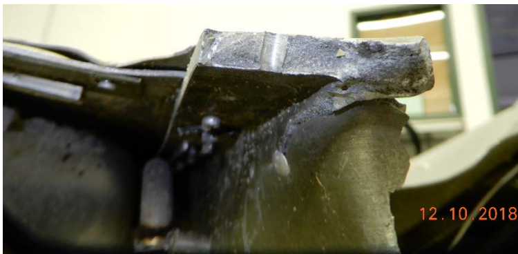
Figure 6: Right Wing Upper Fracture Surface
