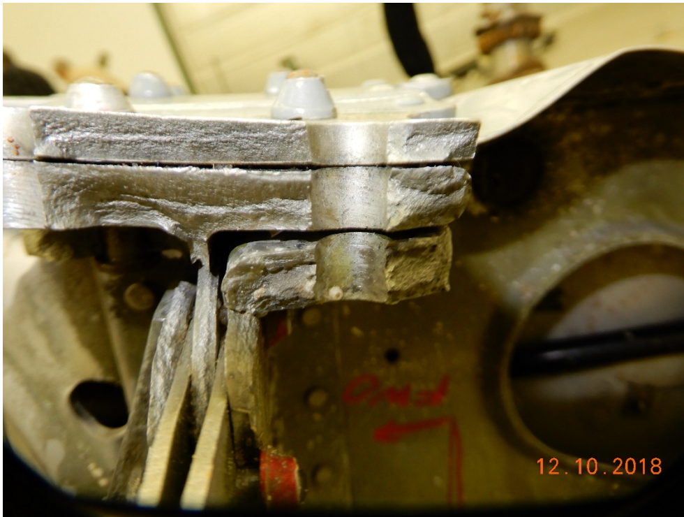
Figure 15: Left Wing Lower fracture Surface
