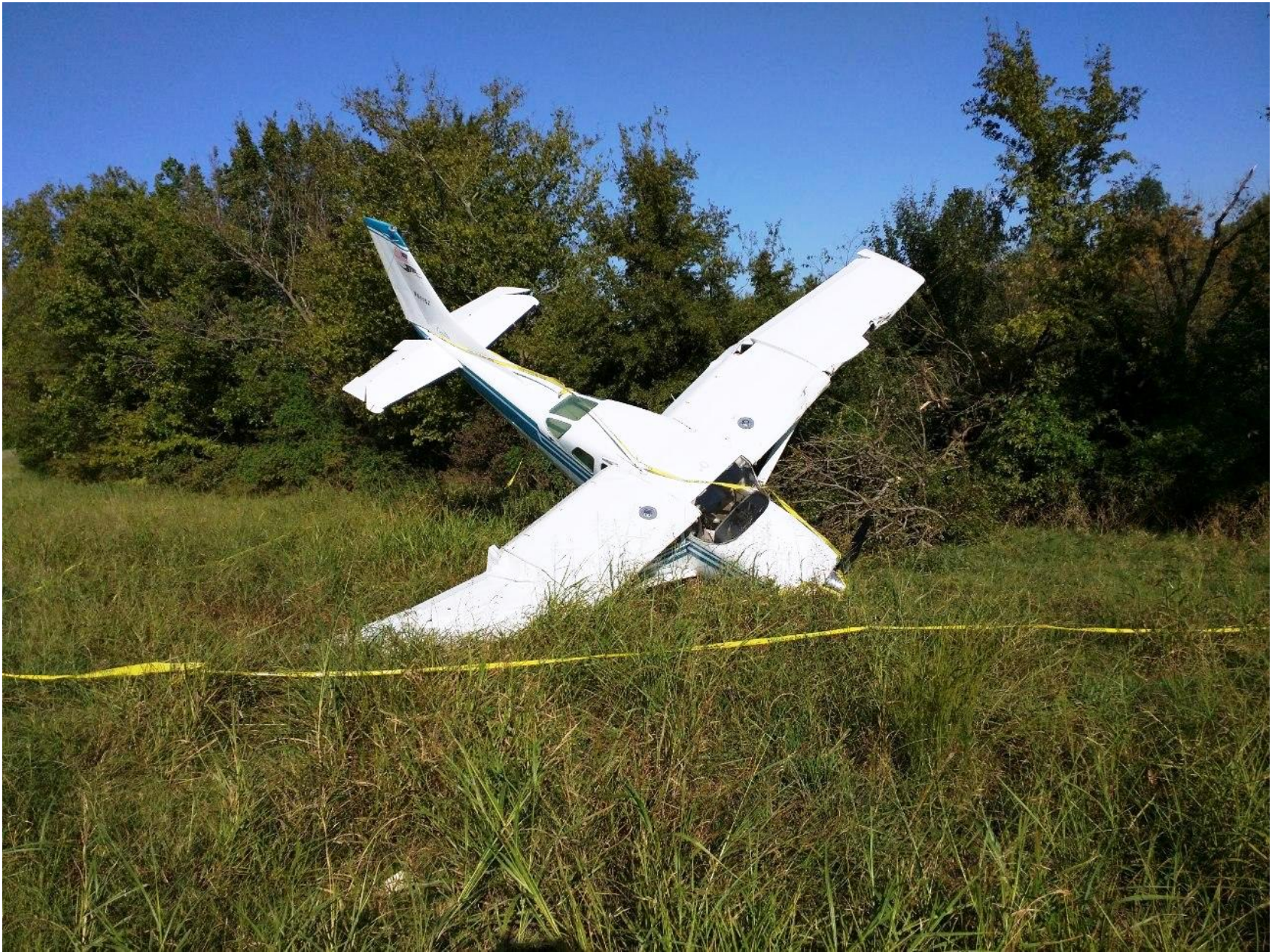
Photo 1 – View of airplane nose down showing buckling damage to right wing
