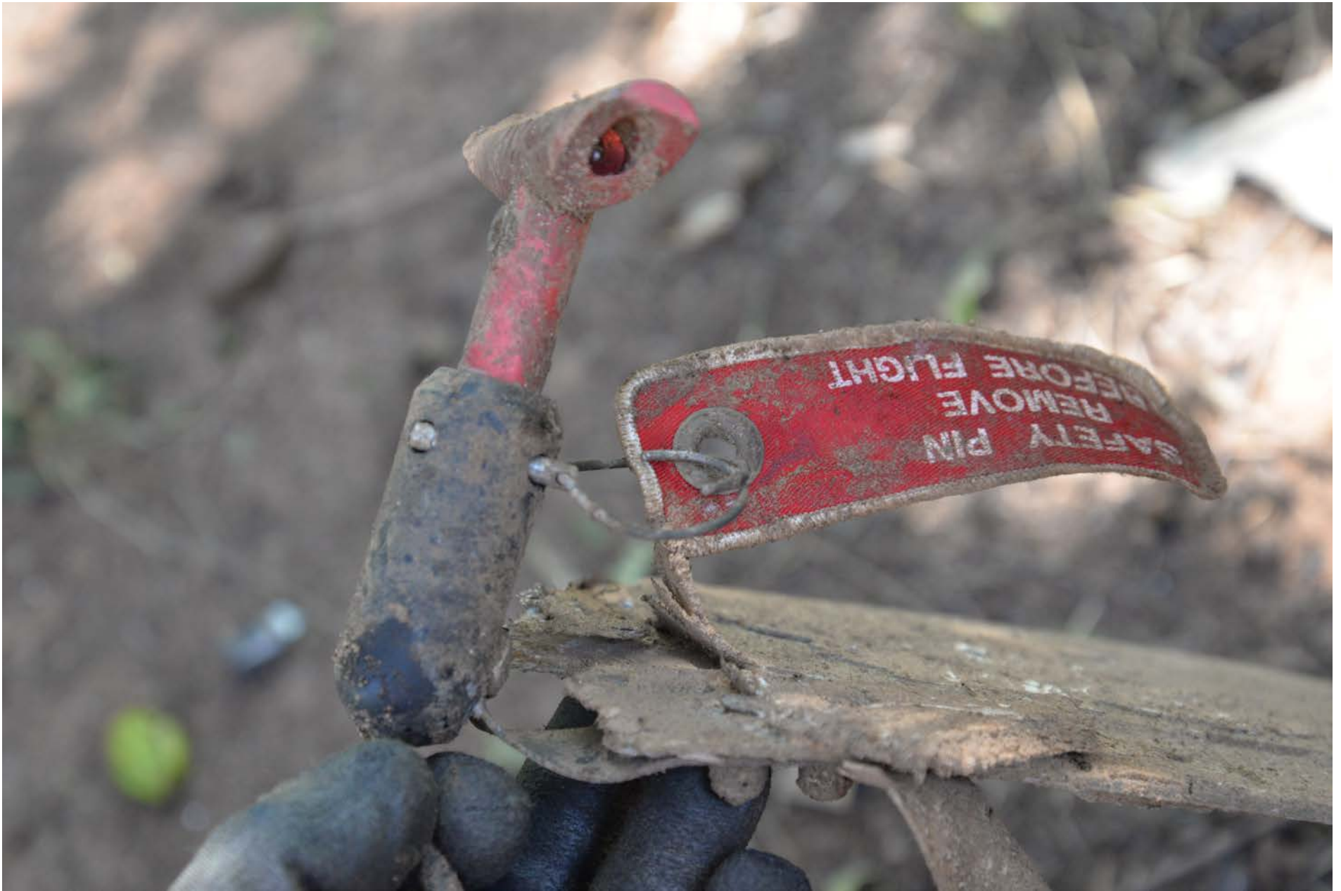
Photo 8 – View of CAPS pin installed in handle. (Courtesy of Cirrus Aircraft)
