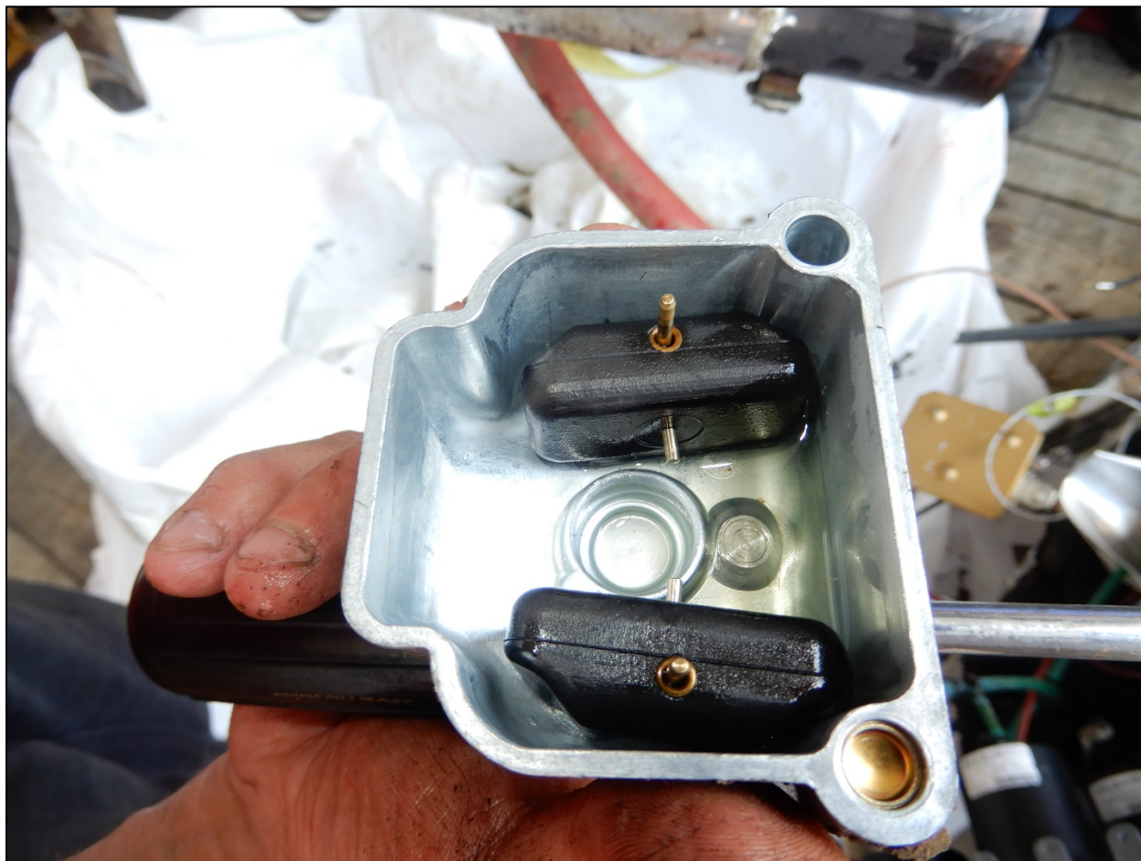
Photo 6: View of the carburetor float bowl with remnants of fuel inside
