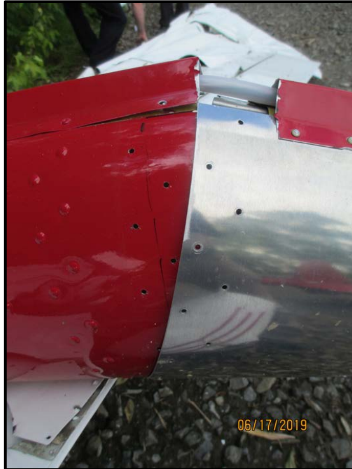
Photograph 18 2 - Right tail boom inboard doubler with separated rivets.
