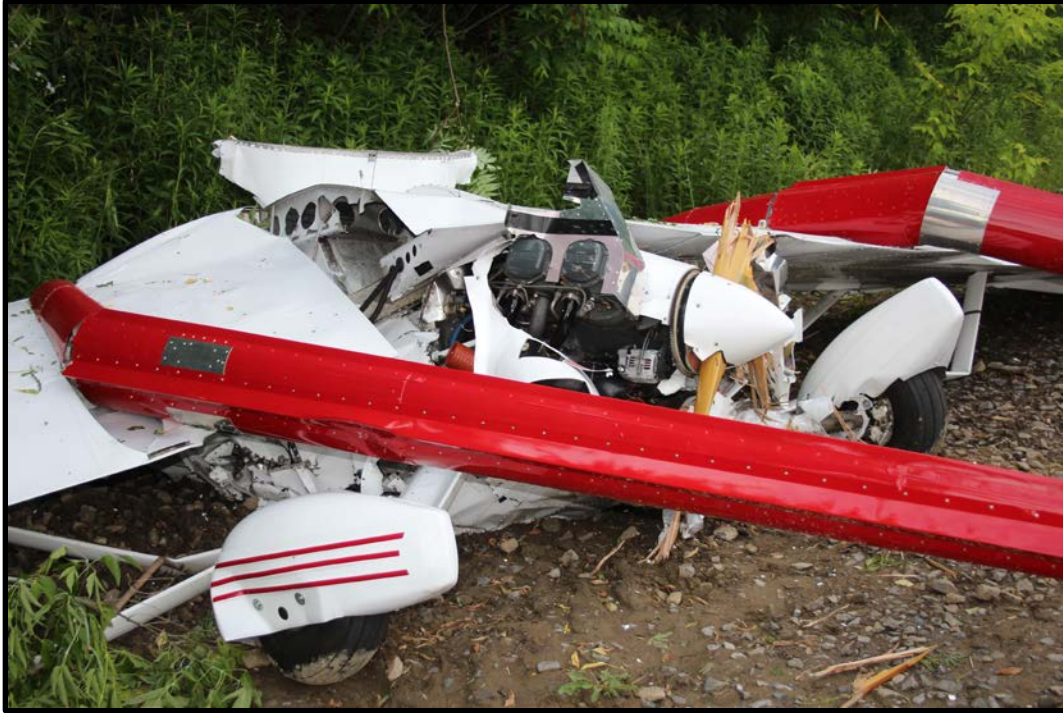
Photograph 14 - Tail booms with external doublers and added stringers.
