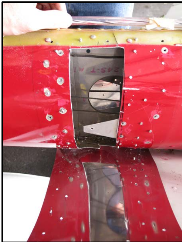
Photograph 17 - Left tail boom inboard hole with cracks.
