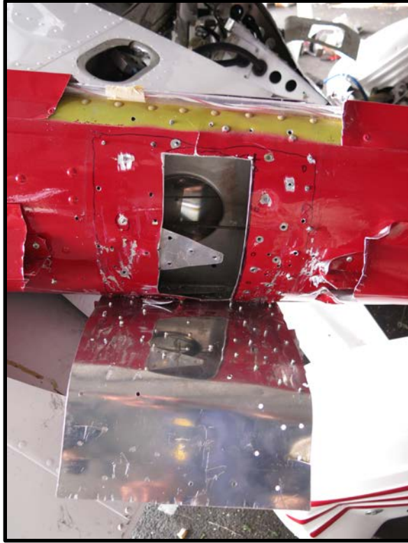
Photograph 16 - Left tail boom outboard hole with cracks.
