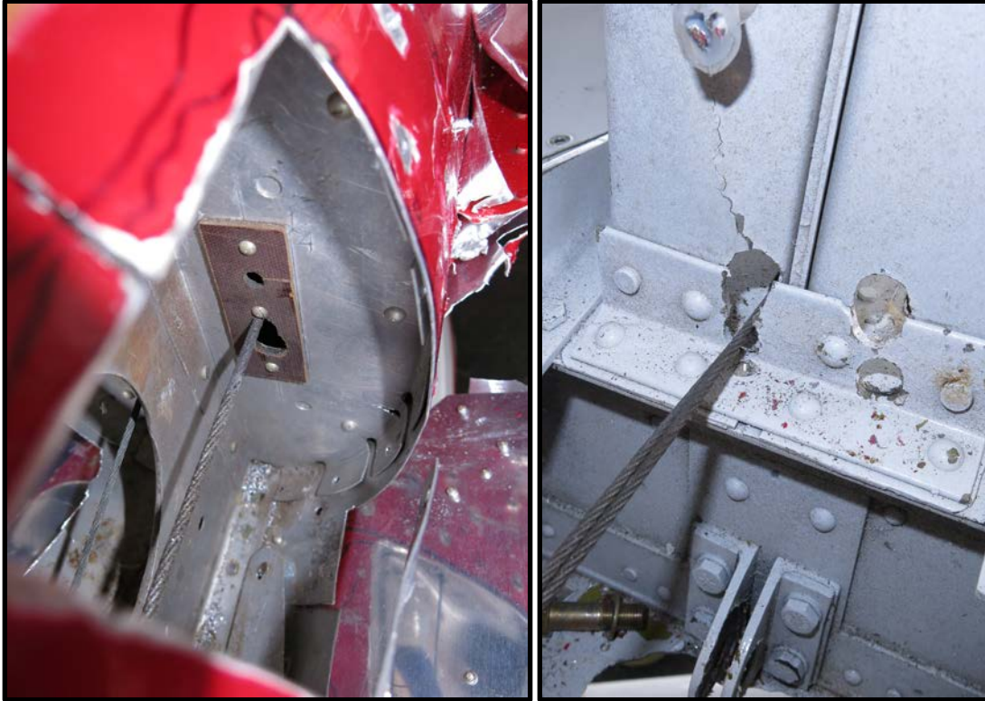
Photograph 19 - Control cable fairlead and pass through.
