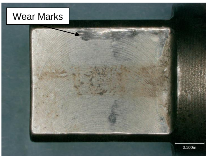
Figure 6. Digital microscope image of the bottom side of the large end of the coupling showing wear marks.
