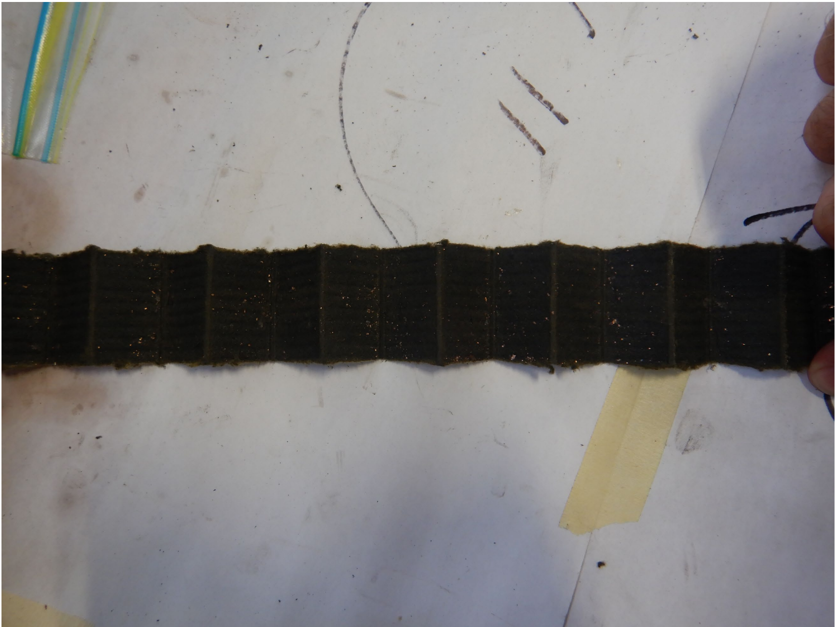
Photo 4 – View of the metallic debris in the oil filter. (Photo courtesy of Textron)
