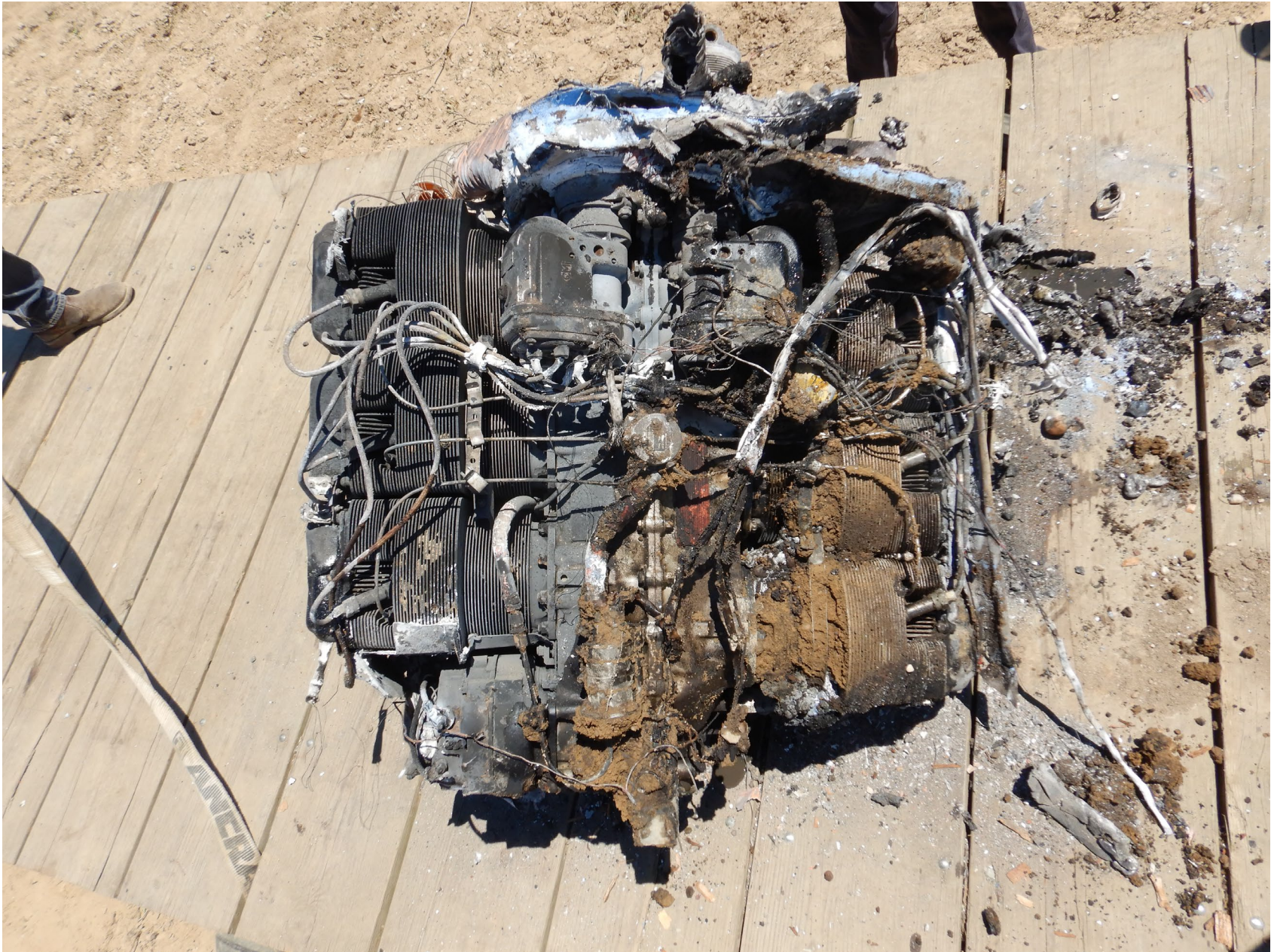
Photo 3 – View of the engine separated from the airframe. (Photo courtesy of Textron)
