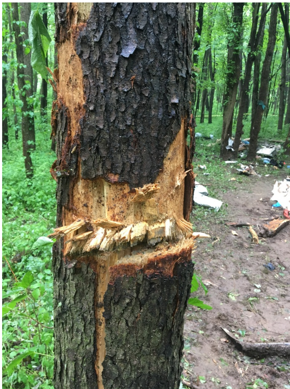
Photo 2 – Propeller Blade Strike in Tree Along Wreckage Path
