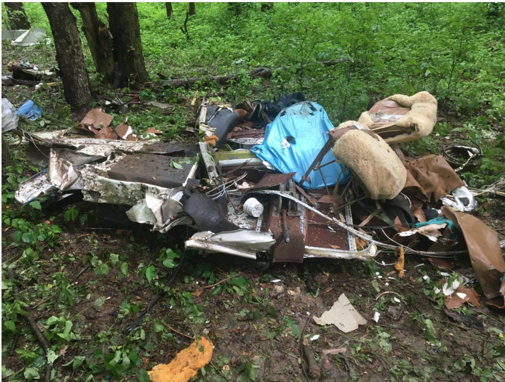
Photo 5 – Main Wreckage Including the Main Cabin Area and Section of Right Wing
