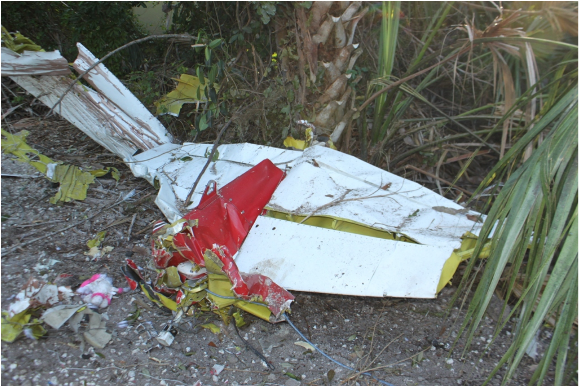
Photo 7 – NTSB Digital Photograph. View Depicting the Separated Empennage.
