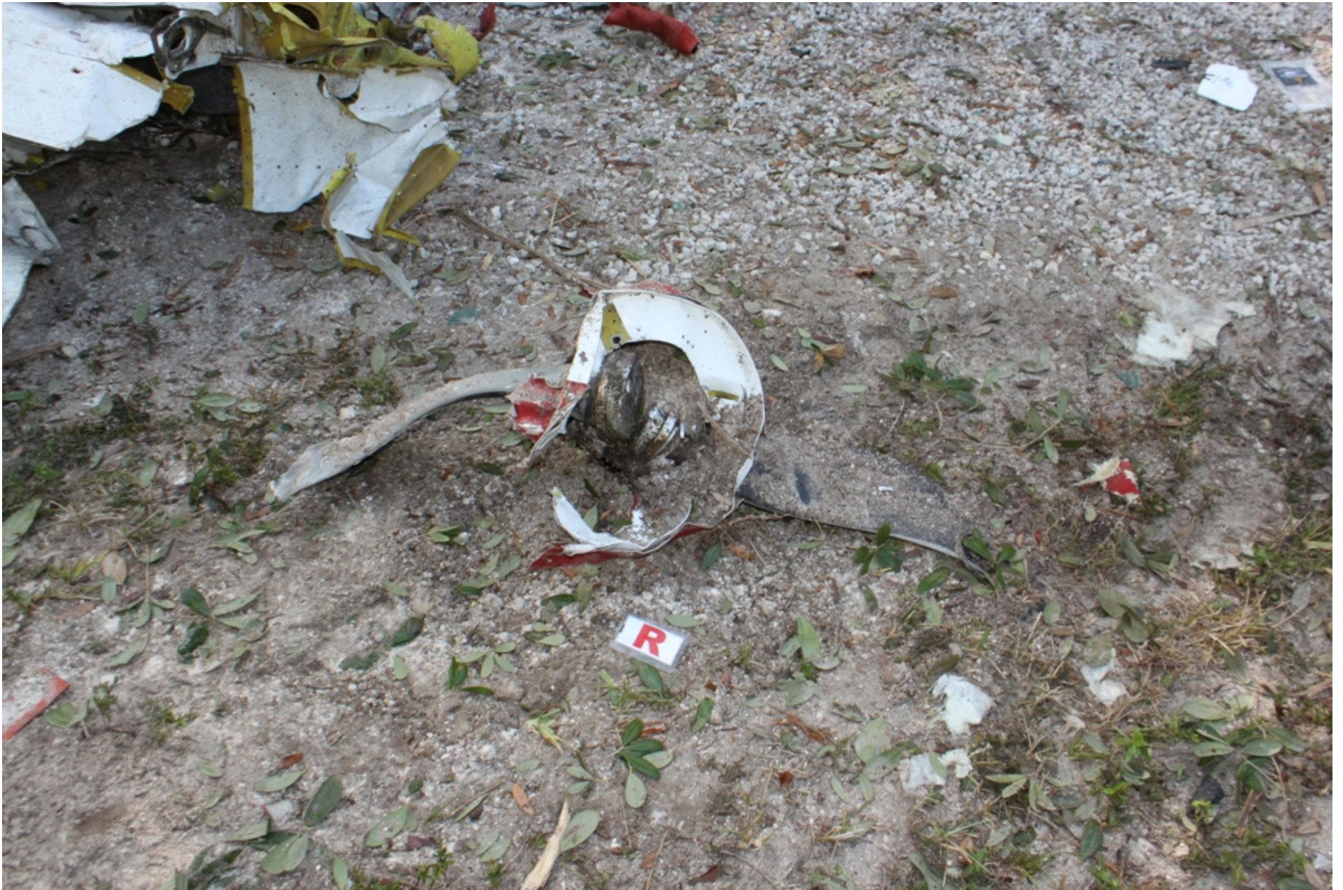
Photo 10 - NTSB Digital Photograph. View Depicting the right Propeller.
