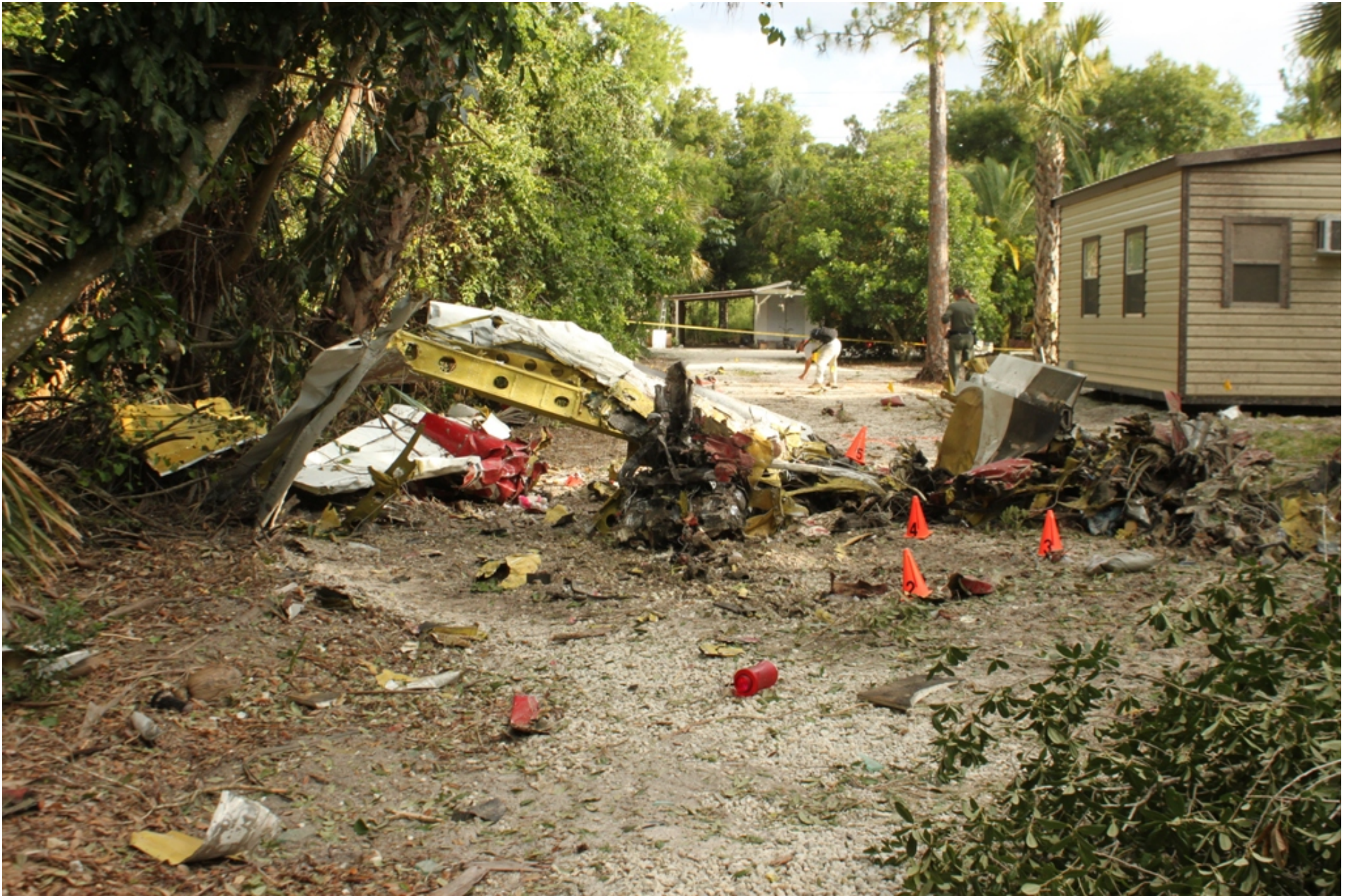
Photo 5 – NTSB Digital Photograph. View Looking in a Southerly Direction. Note the Fragmented Wreckage including Parts of the Wings and Empennage.
