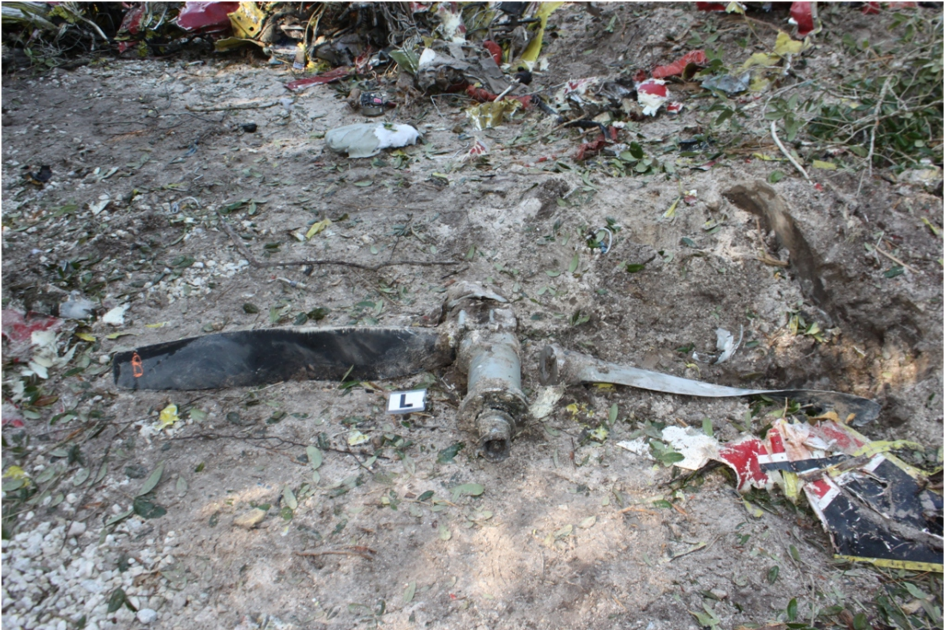
Photo 9 - NTSB Digital Photograph. View Depicting Left Propeller. Note the Blade Bending.
