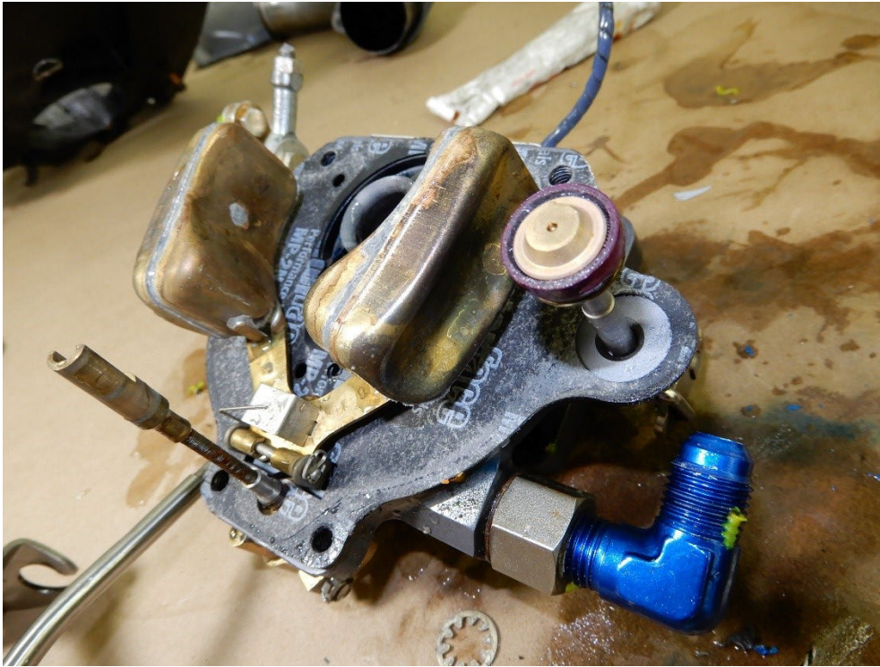
Figure 11. View of disassembled carburetor.
