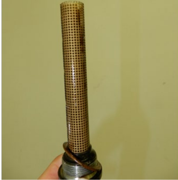
Figure 12. View of oil suction screen.
