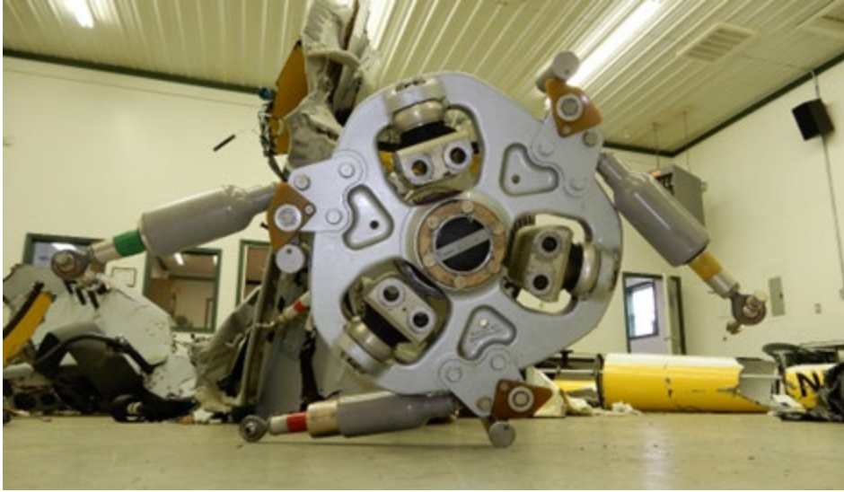
Figure 7. View of rotor head.
