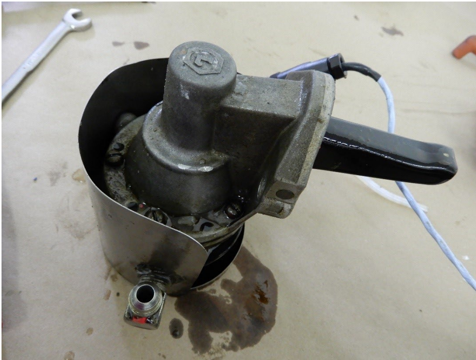
Figure 13. View of mechanical fuel pump.
