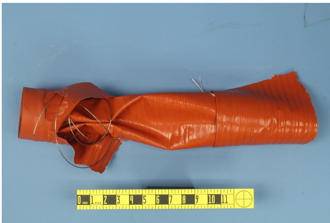
Figure 4: Images of the SCEET tube from the accident vehicle after dissection: a) side view from one direction and b) side view from the opposing direction.
