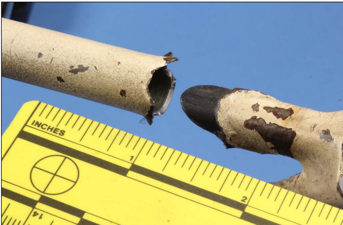
Figure 2. Closer view of the fracture in the lower arm of the left upper engine mount.
