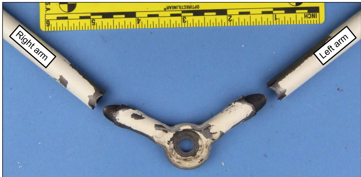
Figure 13. Lower side of the lower mount as viewed looking upward and aft photographed after cracks had been opened by lab fracture.
