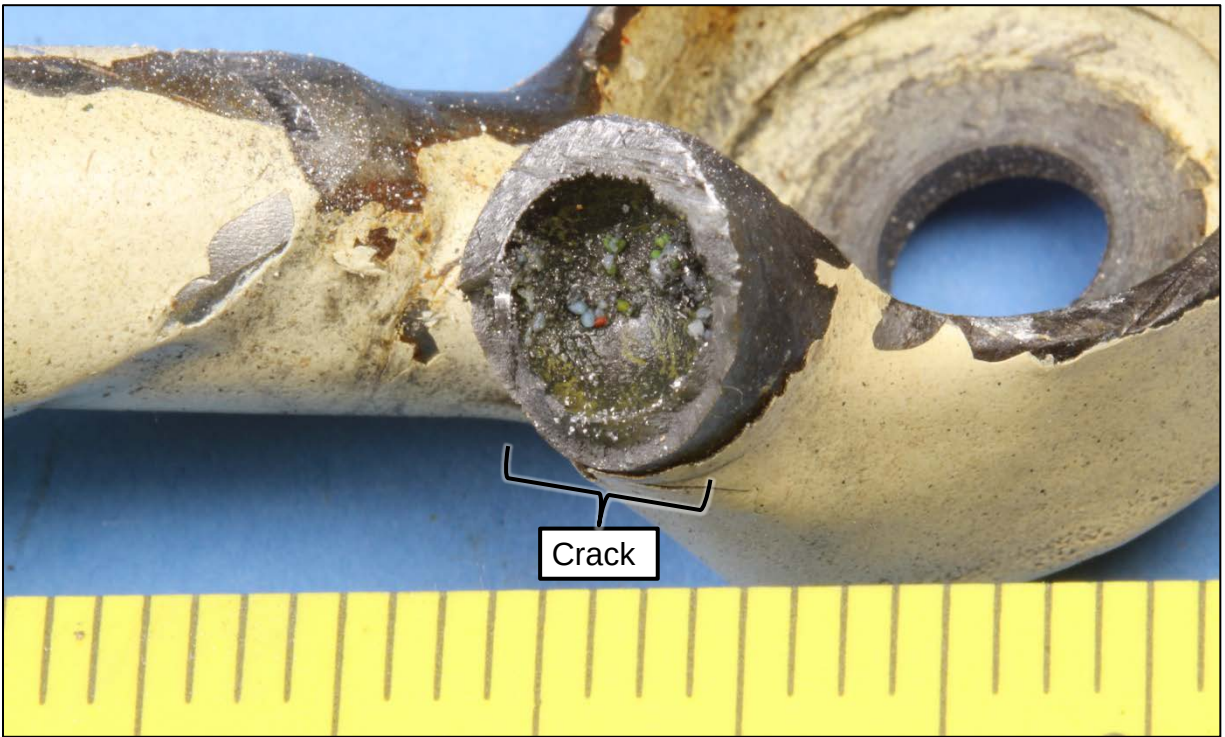
Figure 15. Fracture features of the crack in the upper arm of the right upper engine mount photographed after the crack was opened in the lab.
