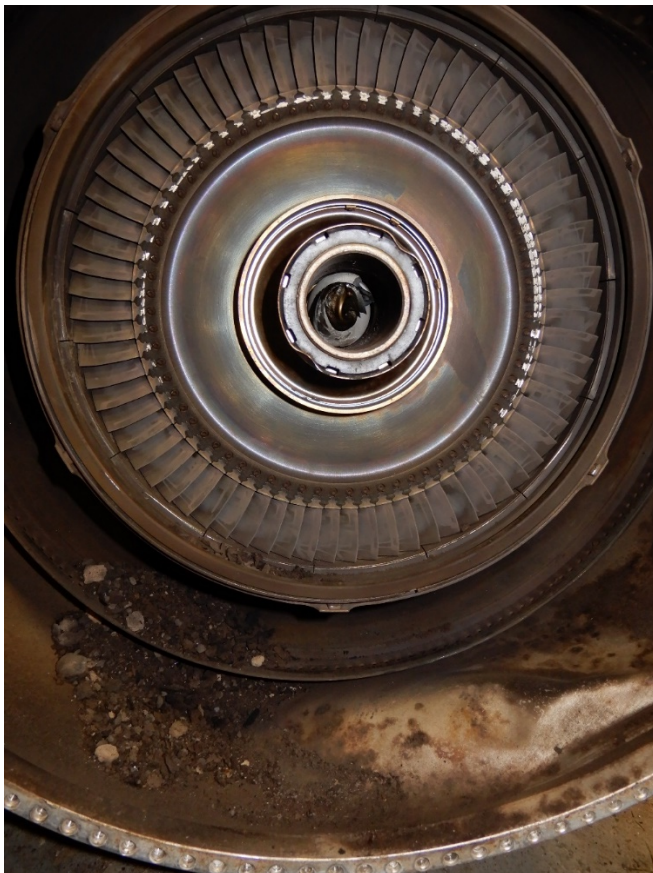
Figure 11. Trailing edge view of first stage turbine. Note debris inside engine and rotational scoring on turbine.
