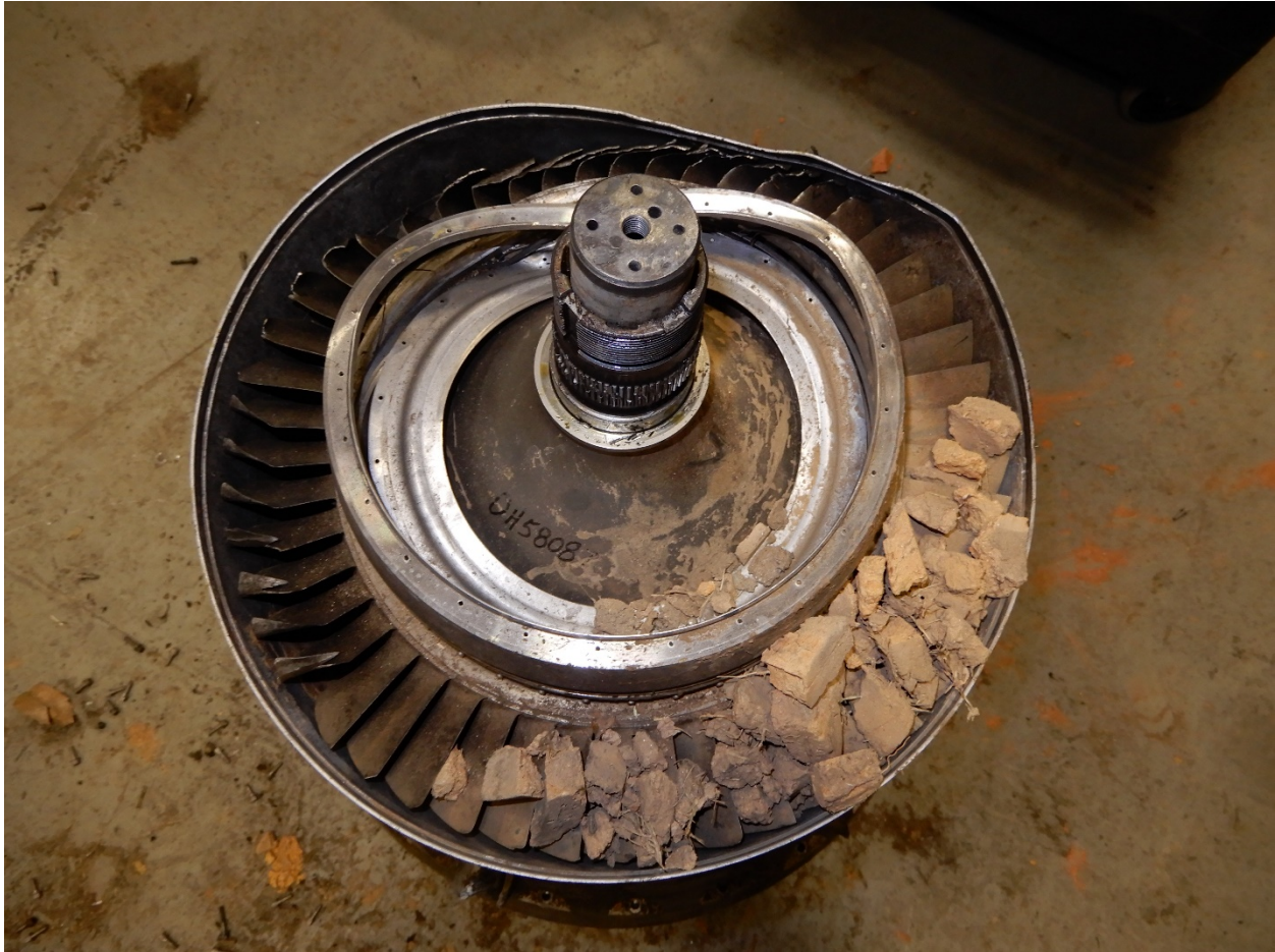
Figure 12. View of boost turbine. Note blades bent the opposite direction of travel.
