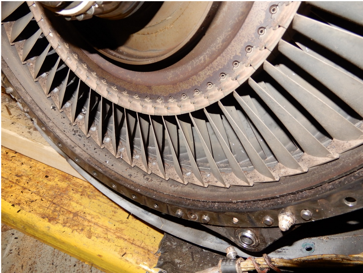
Figure 5. Trailing edge view of third stage turbine. Note debris and rotational scoring.
