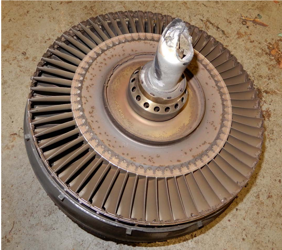
Figure 6. View of second stage turbine and separate shaft.
