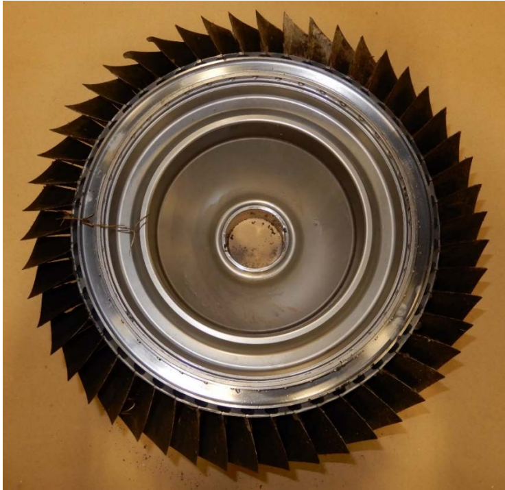
Figure 4. Trailing edge view of boost turbine.
