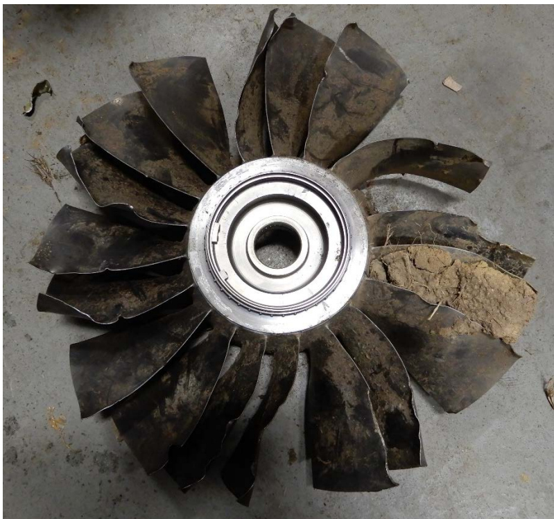
Figure 3. View of right fan with all blades bent the opposite direction of travel.
