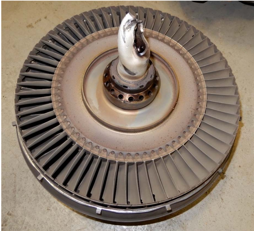
Figure 10. View of left engine shaft fracture.
