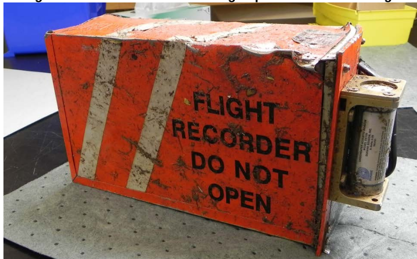
Figure 1. Exterior of CVR showing impact structural damage.
