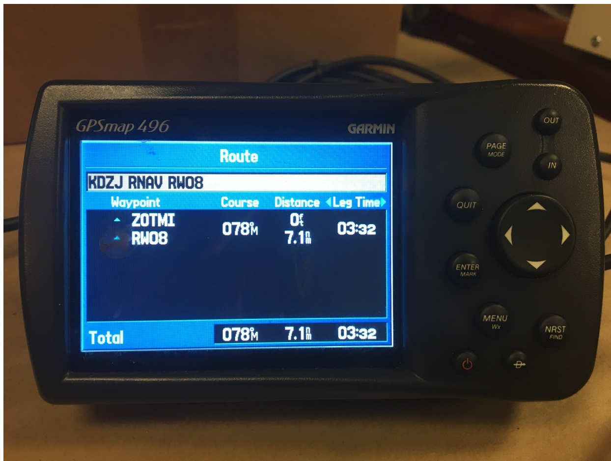
Figure 7. View of KDZJ RNAV RW08 route programed into GPS.
