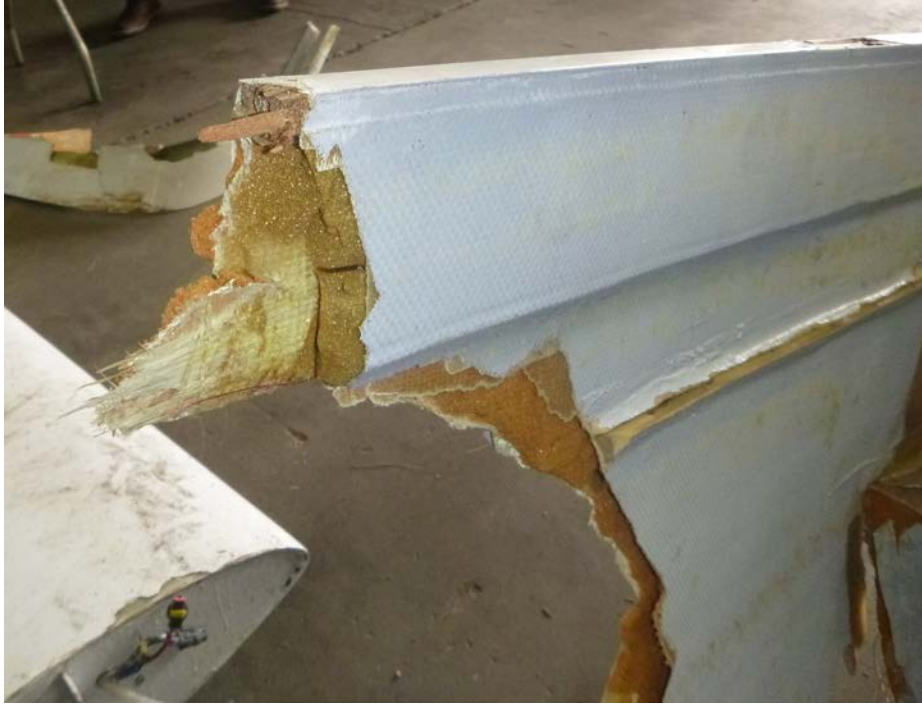
Figure 3 – Left longeron fracture, forward fuselage section
