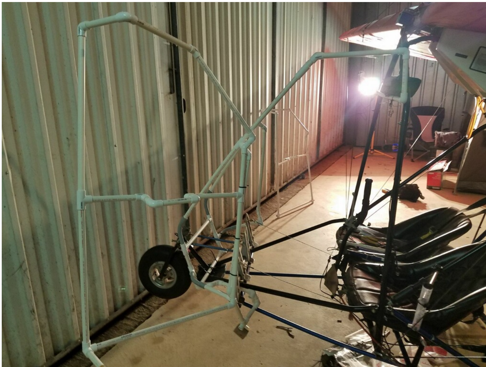
Photo 6 – View of PVC-Tubing Frame for Cockpit Enclosure Secured with Zip-Ties
