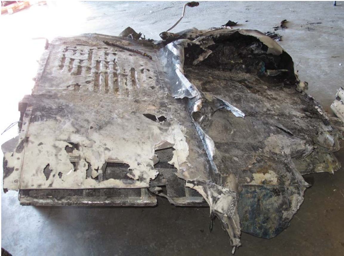
Figure 9. Upper surface of right engine nacelle.
