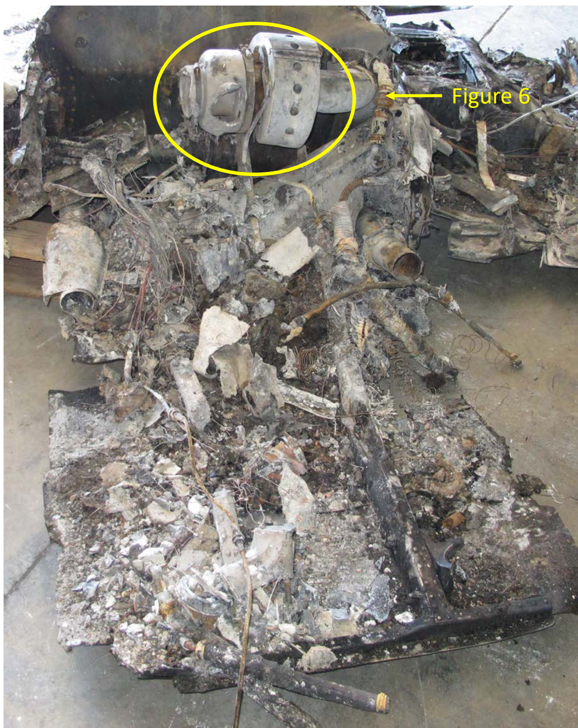
Figure 5. Left engine lower nacelle and cowling.
