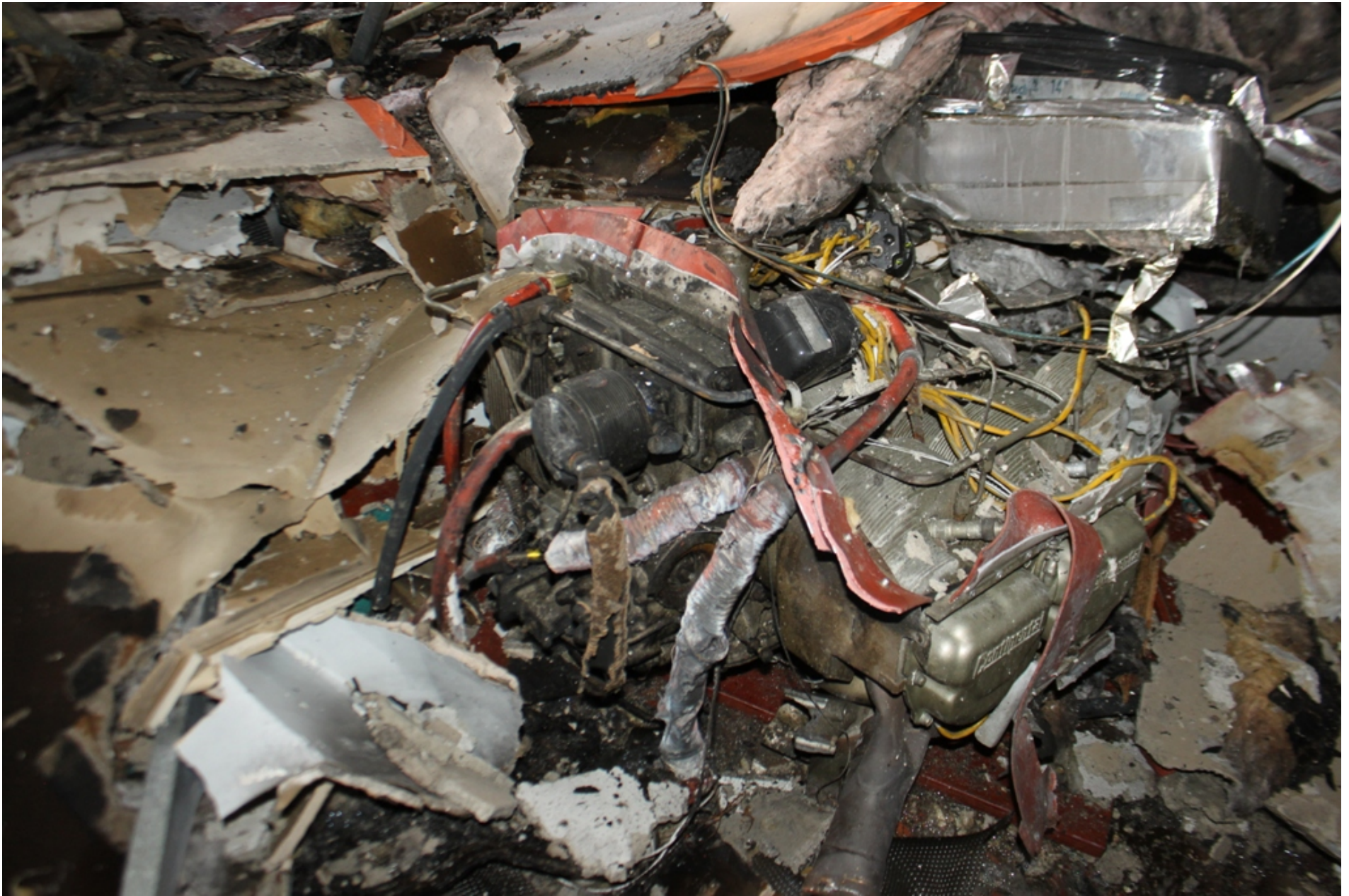
Photo 11 - NTSB Digital Photograph. View of the Rear Portion of the Right Engine Assembly Before Recovery From the Impacted Building.
