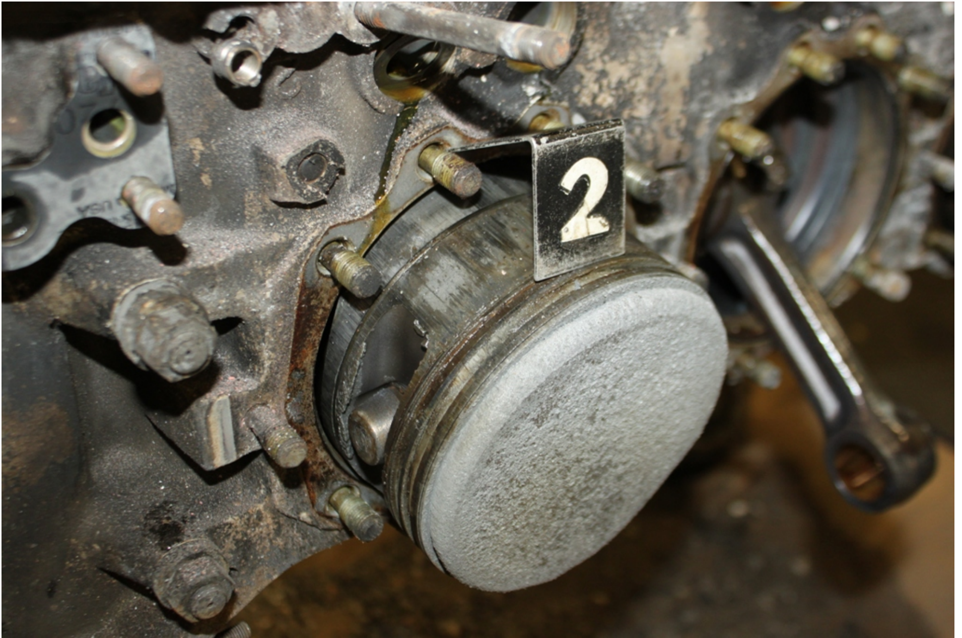
Photo 19 - NTSB Digital Photograph. View of the No. 2 Piston. Note the Damage to the Crown.
