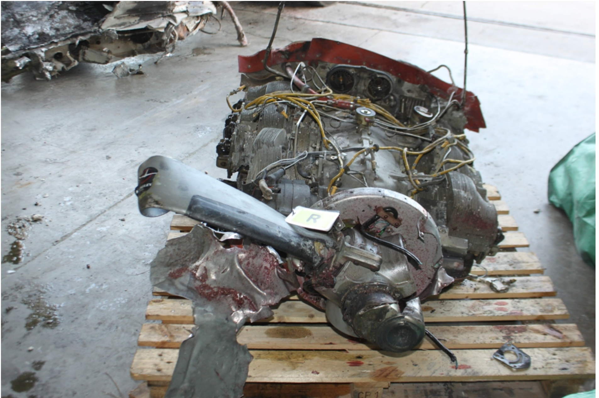
Photo 13 - NTSB Digital Photograph. View of the Right Engine with Attached Propeller Following Recovery from the Impacted Building. Note the Separated Propeller Blades.
