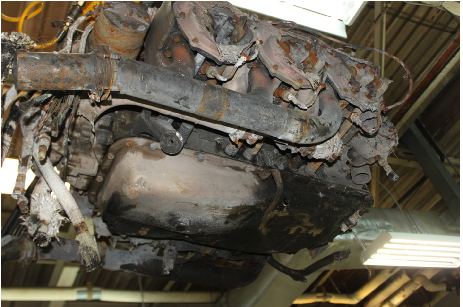
Photo 15 - NTSB Digital Photograph. View of the Bottom of the Left Engine Assembly. Note the Discoloration of a Portion of the Exhaust for the Nos. 2, 4, and 6 Cylinders in the Background Compared to the Exhaust for the Nos. 1, 3, and 5 Cylinders in the Foreground.
