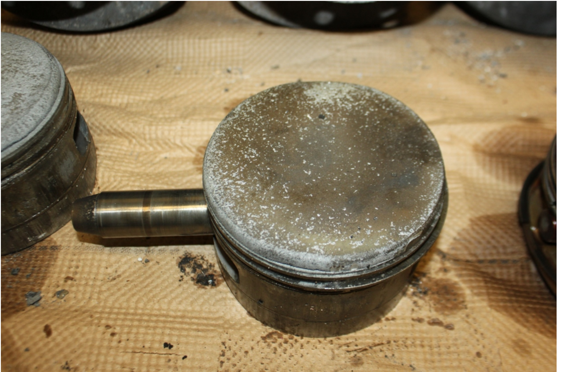
Photo 20 - NTSB Digital Photograph. View of the No. 3 Piston. Note the Damage to the Crown.
