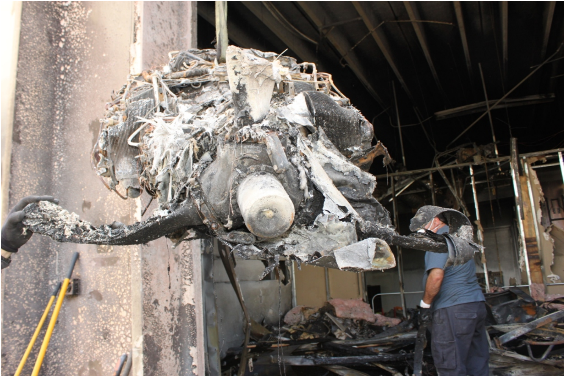
Photo 10 - NTSB Digital Photograph. View of the Left Engine Assembly With Attached Propeller During Recovery From Building. Note the Extensive Fire Damage.
