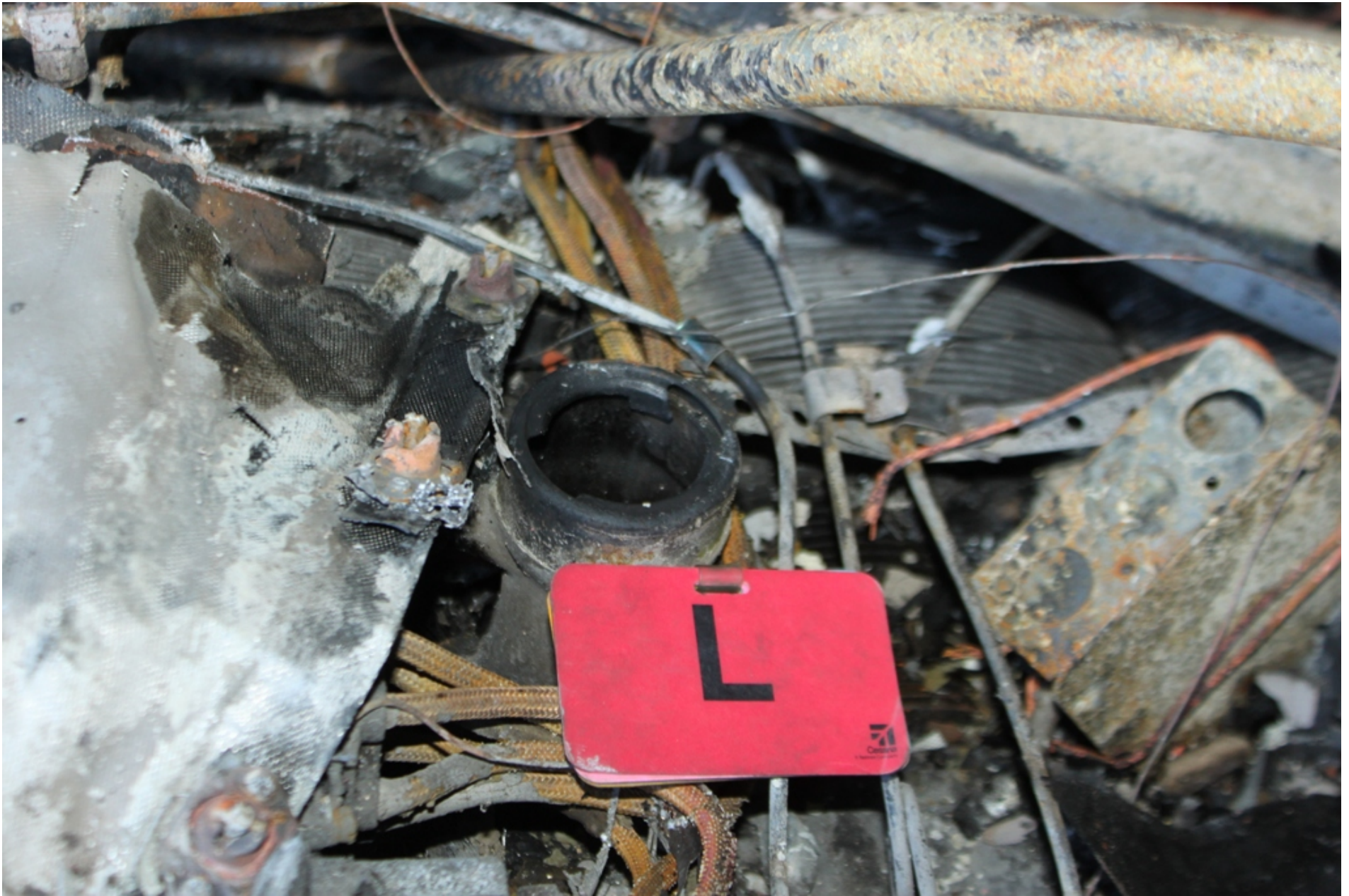
Photo 9 - NTSB Digital Photograph. View of the Left Engine Breather Assembly. Note the Missing Rod-Oil Gauge and Cap Assembly.
