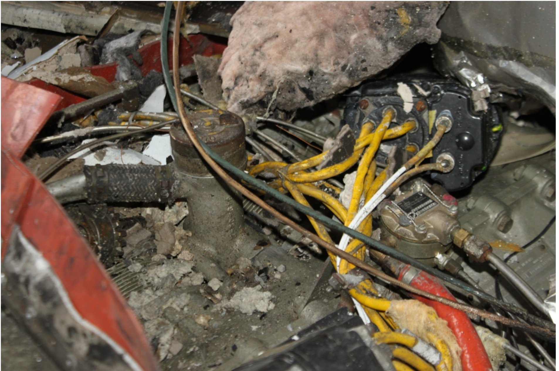
Photo 12 - NTSB Digital Photograph. View of the Right Engine Breather Assembly and Attached Rod-Oil Gauge and Cap Assembly.
