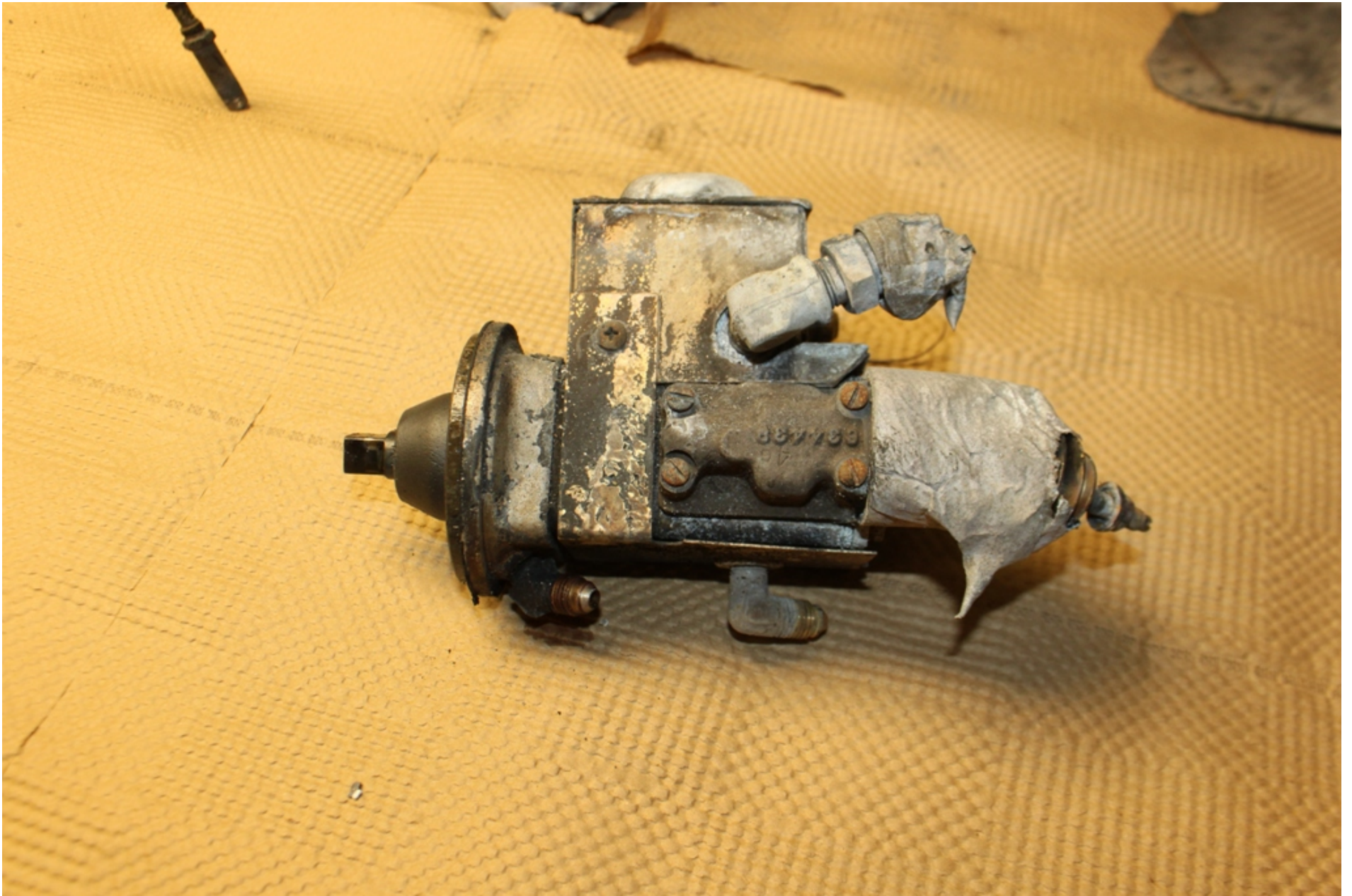
Photo 18 - NTSB Digital Photograph. View of the Left Engine-Driven Fuel Pump. Note the Extensive Heat Damage.
