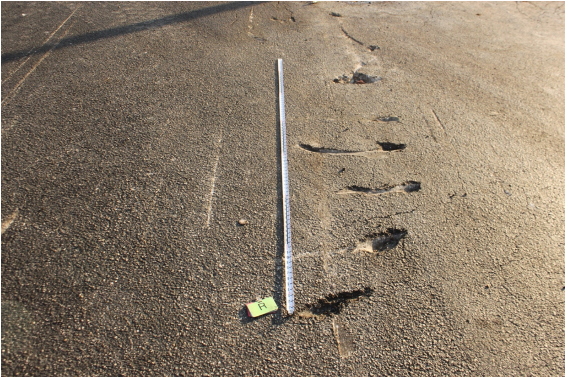
Photo 7 - NTSB Digital Photograph. View of the Ground Scars From Right Propeller. Note the Close Spacing Between the First and Second Which Measured About 10 Inches.
