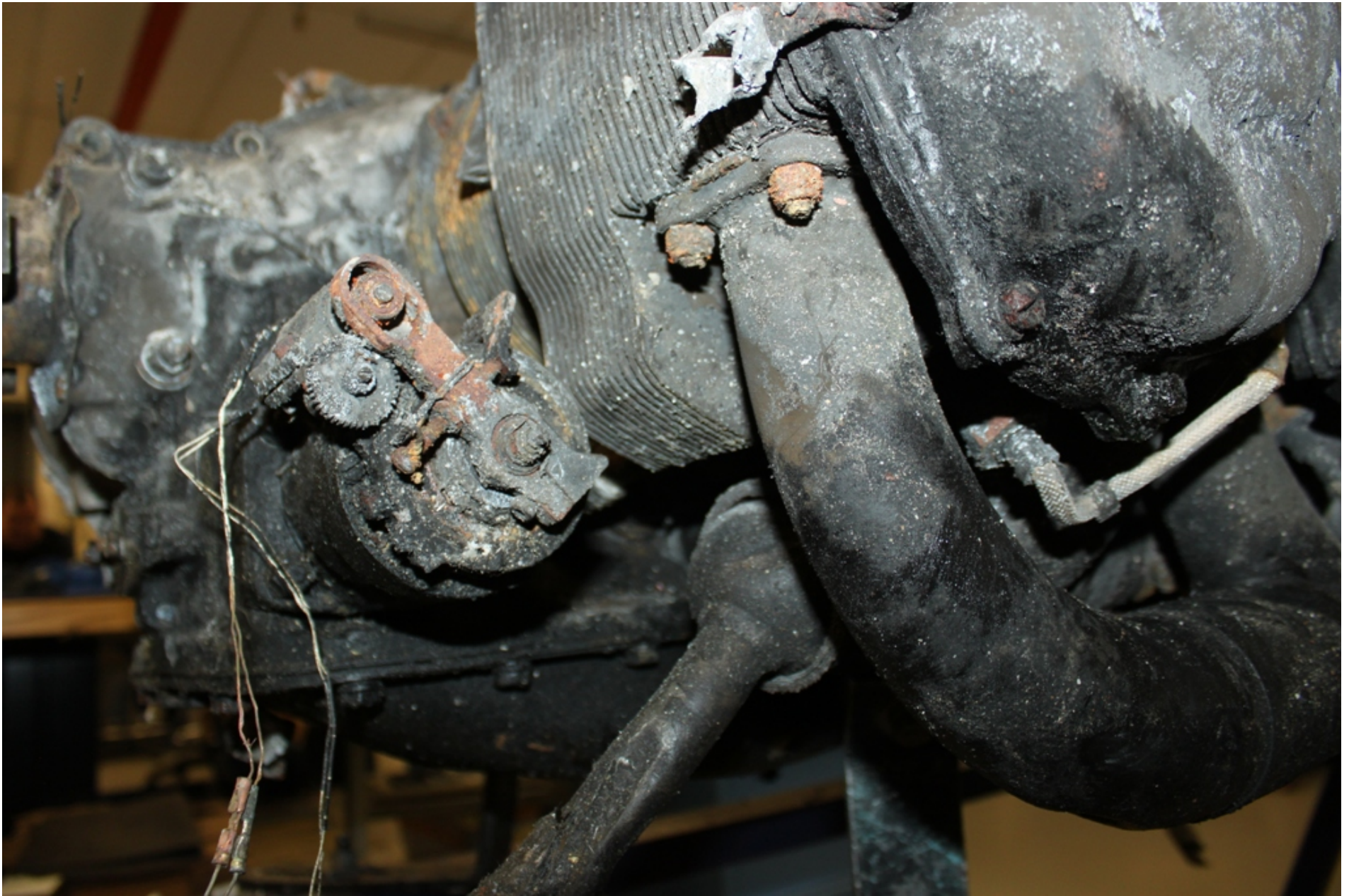
Photo 16 - NTSB Digital Photograph. View of the Heat Damaged Left Propeller Governor. Note the Staining on the Adjacent Section of Exhaust.
