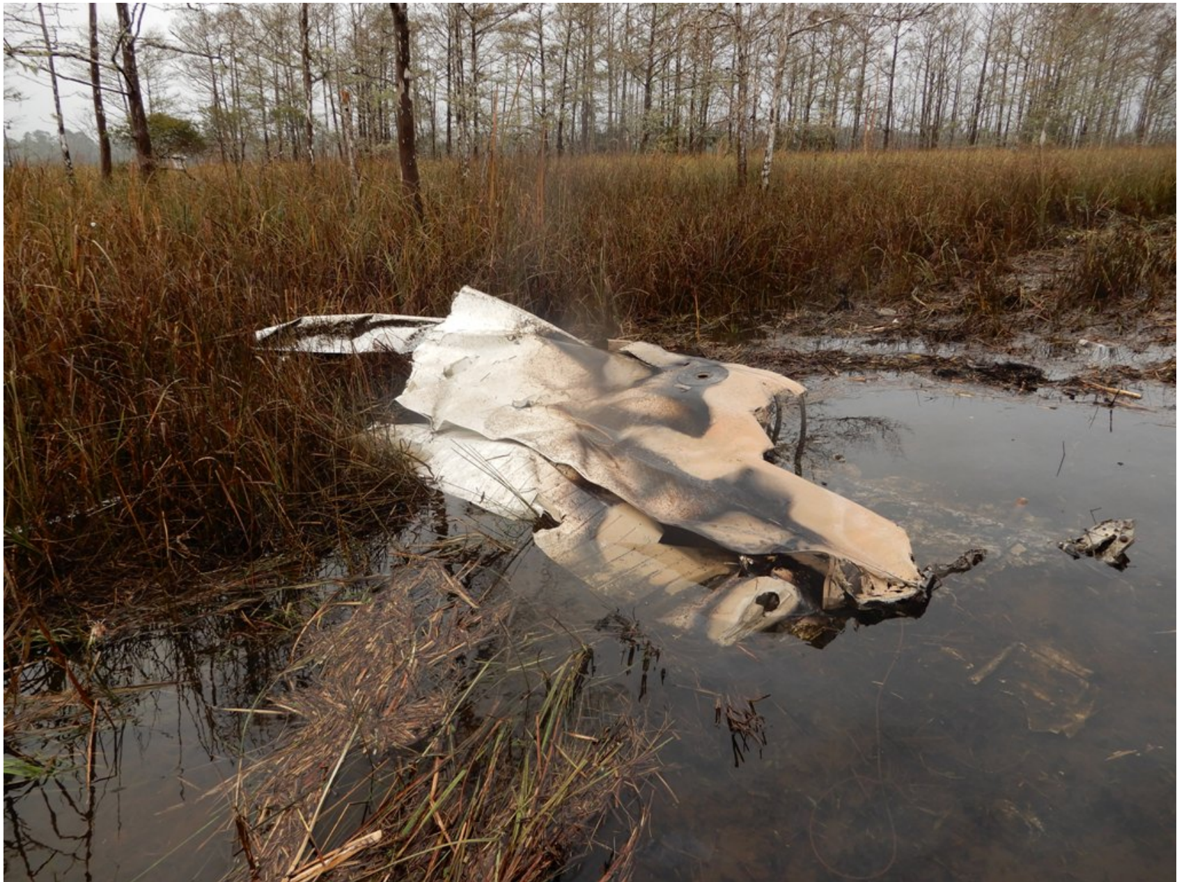
Photo 3 – Right Wing Section (NTSB Photo)
