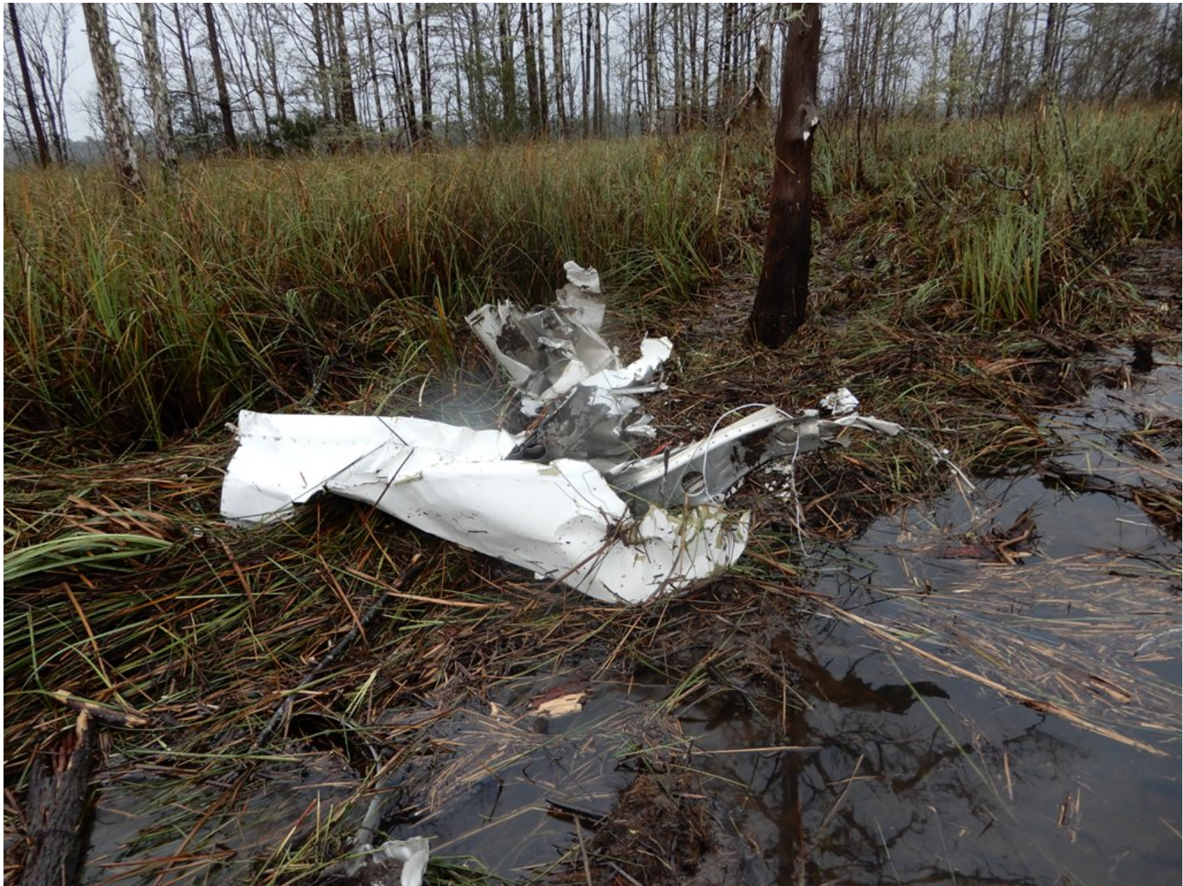
Photo 5 - Right Wing Section (NTSB Photo)
