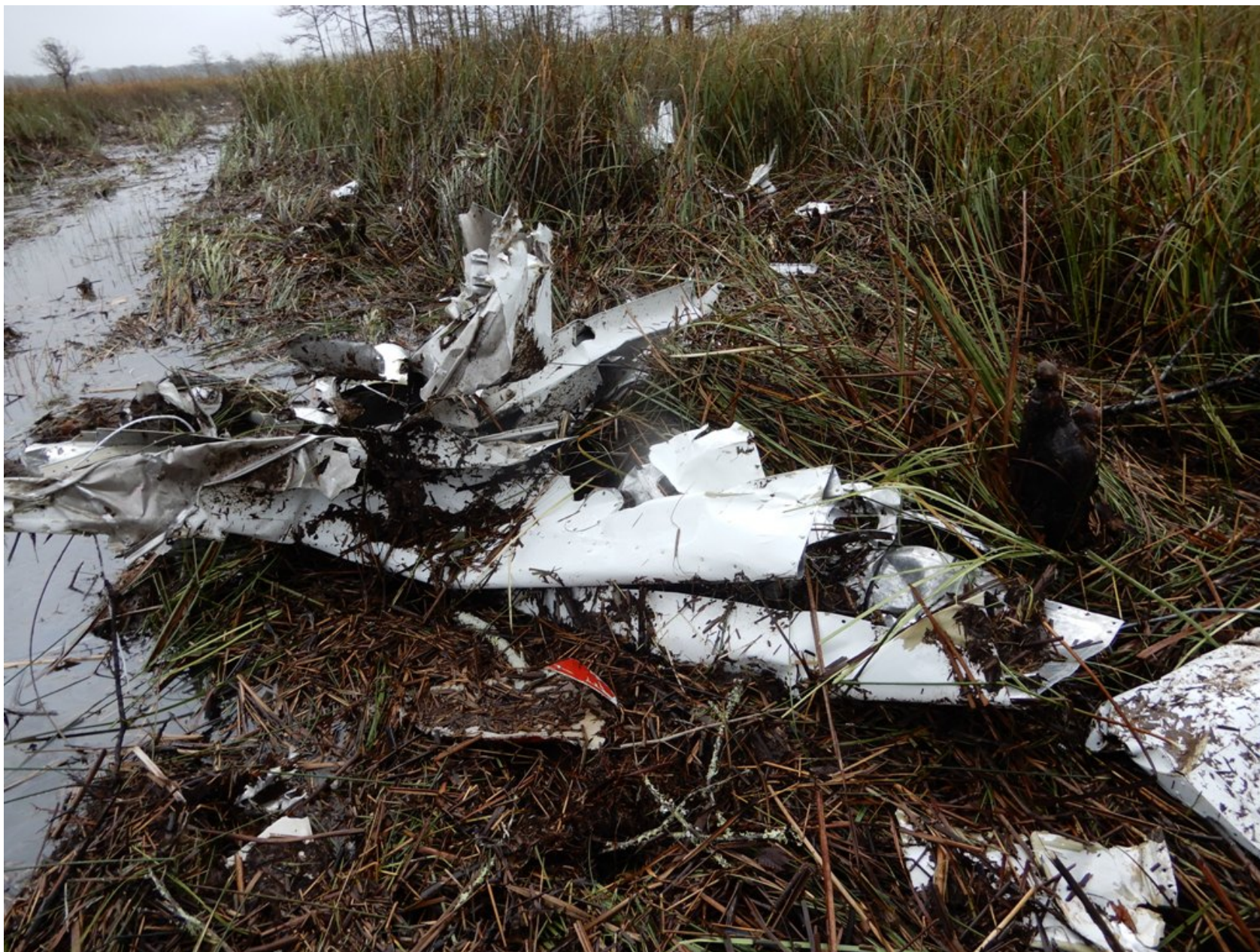
Photo 6 - Left Wing Section (NTSB Photo)
