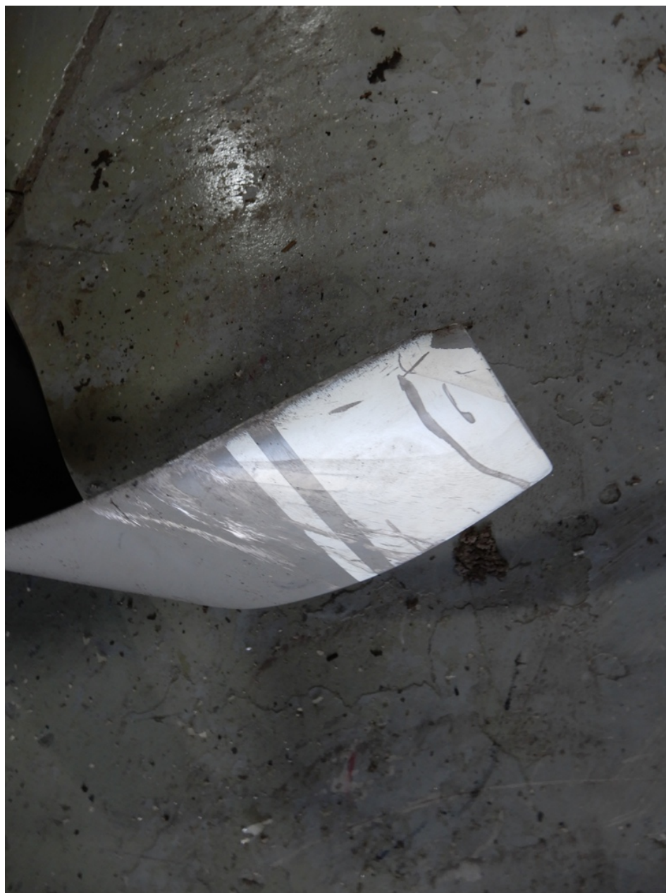
Photo 13 - Propeller Blade Damage (NTSB Photo)
