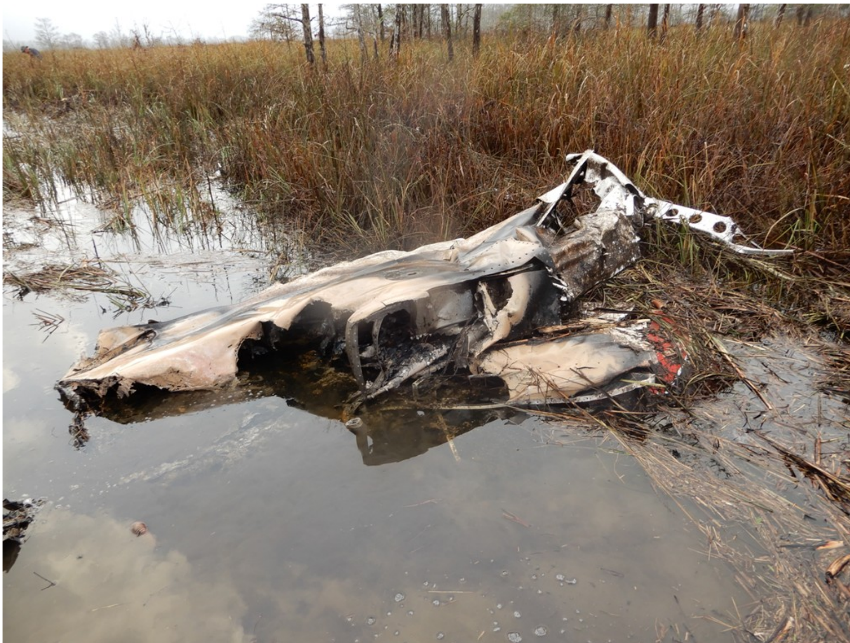
Photo 4 - Right Wing Section (NTSB Photo)
