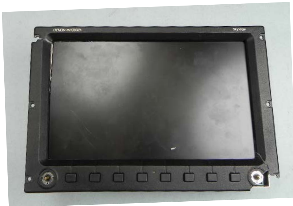
Figure 1. Damaged exterior of flight recorder.
