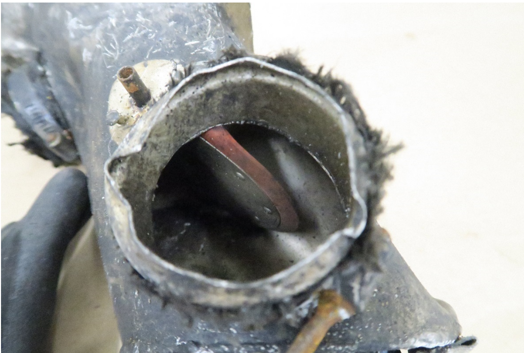
Heater internal flapper valve, TAI Wreckage Exam, ADI-18-DK-029
