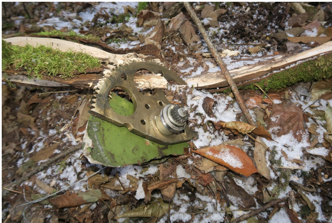
Portion of landing gear gearbox, TAI On-site ASI-DK-055
