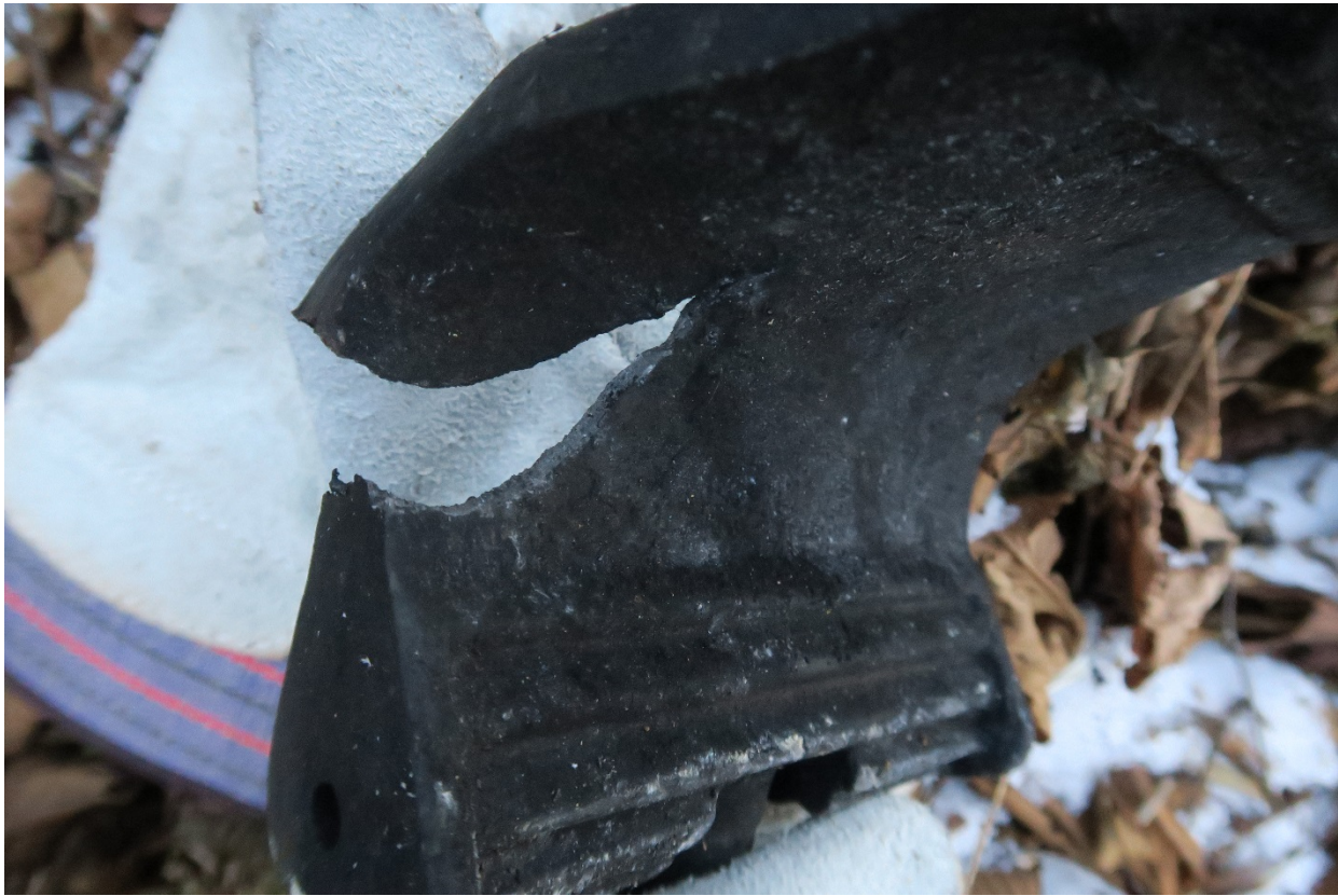
Pilot left rudder pedal, TAI On-site ASI-DK-194
