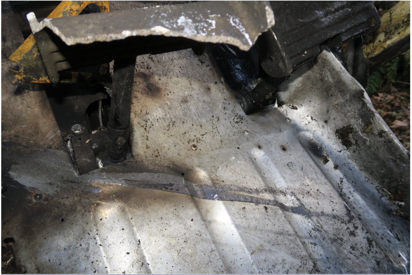
Co-pilot LH rudder pedal, TAI On-site ASI-DK-154
