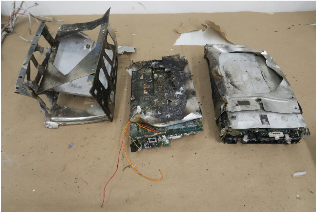
Comm/Nav unit with localized thermal damage, TAI Wreckage Review, ASI-18-DK-032
