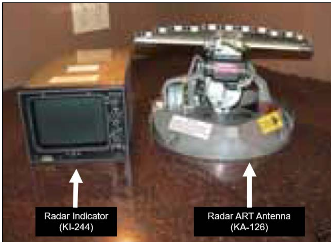
Figure 1: Exemplar Radar Display and Antenna
