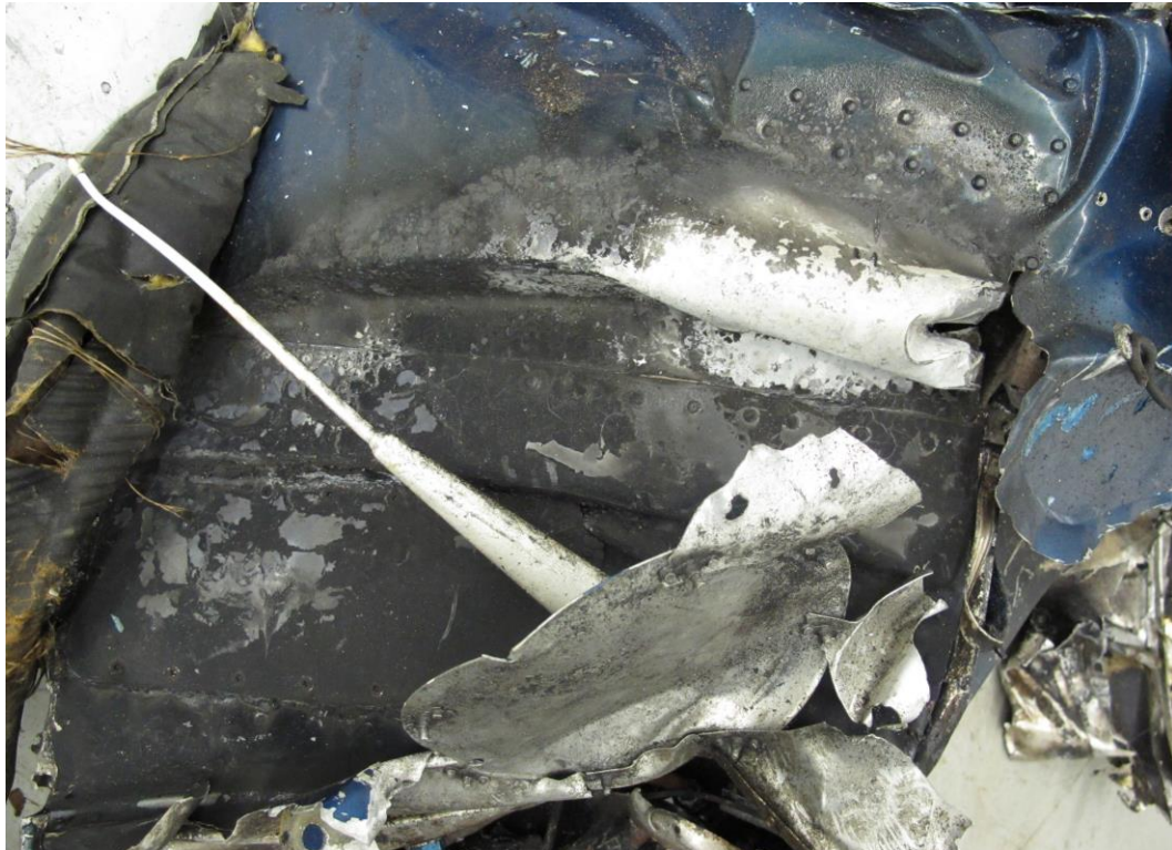
Figure 6. Exterior fuselage surface located under cockpit floor.
