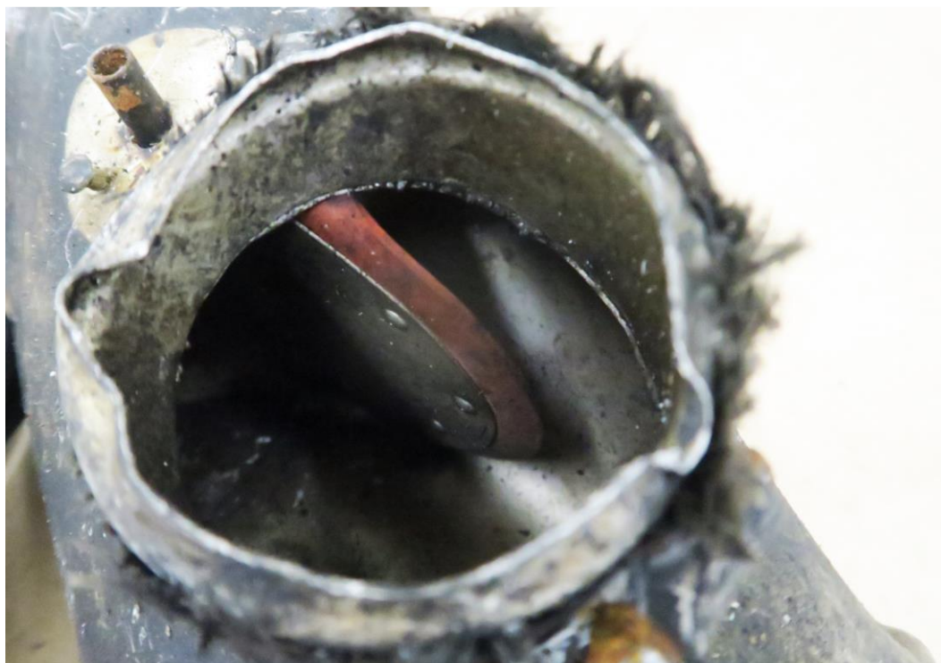
Figure 19. Air control flapper valve inside the cabin heater.
