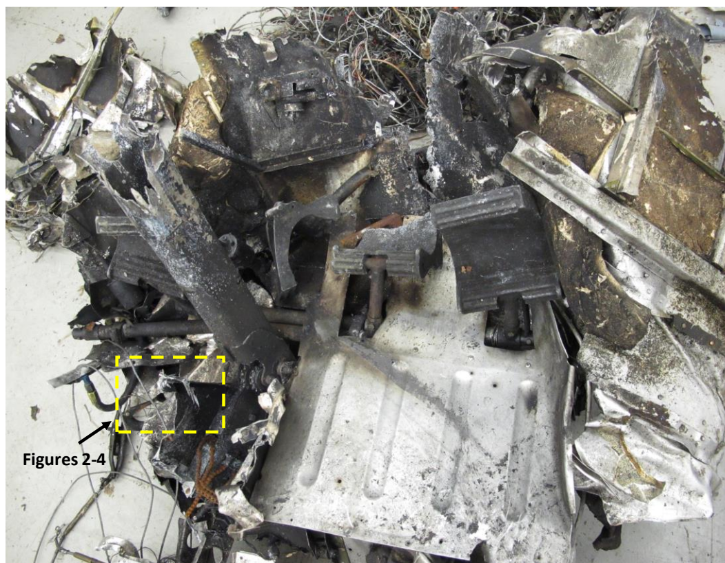
Figure 1. Recovered section of cockpit floor
