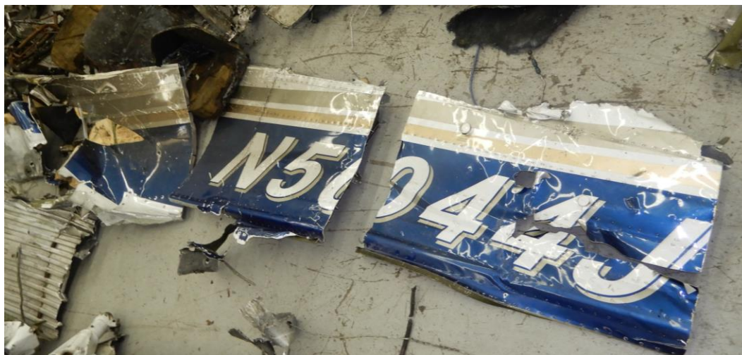
Figure 11. Section of fuselage (left side).
