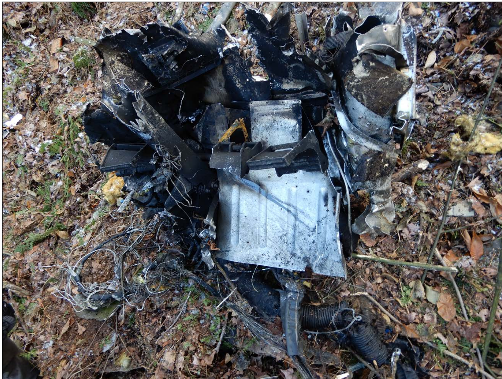
Photo 5: Fragment of the floor of the cockpit section
