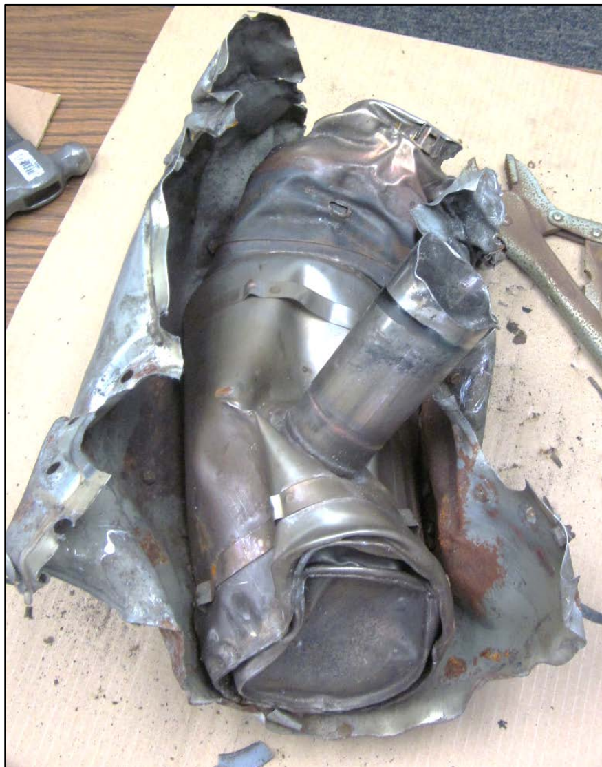
Photo 3: View of Heater with Outer Shroud Peeled Back
