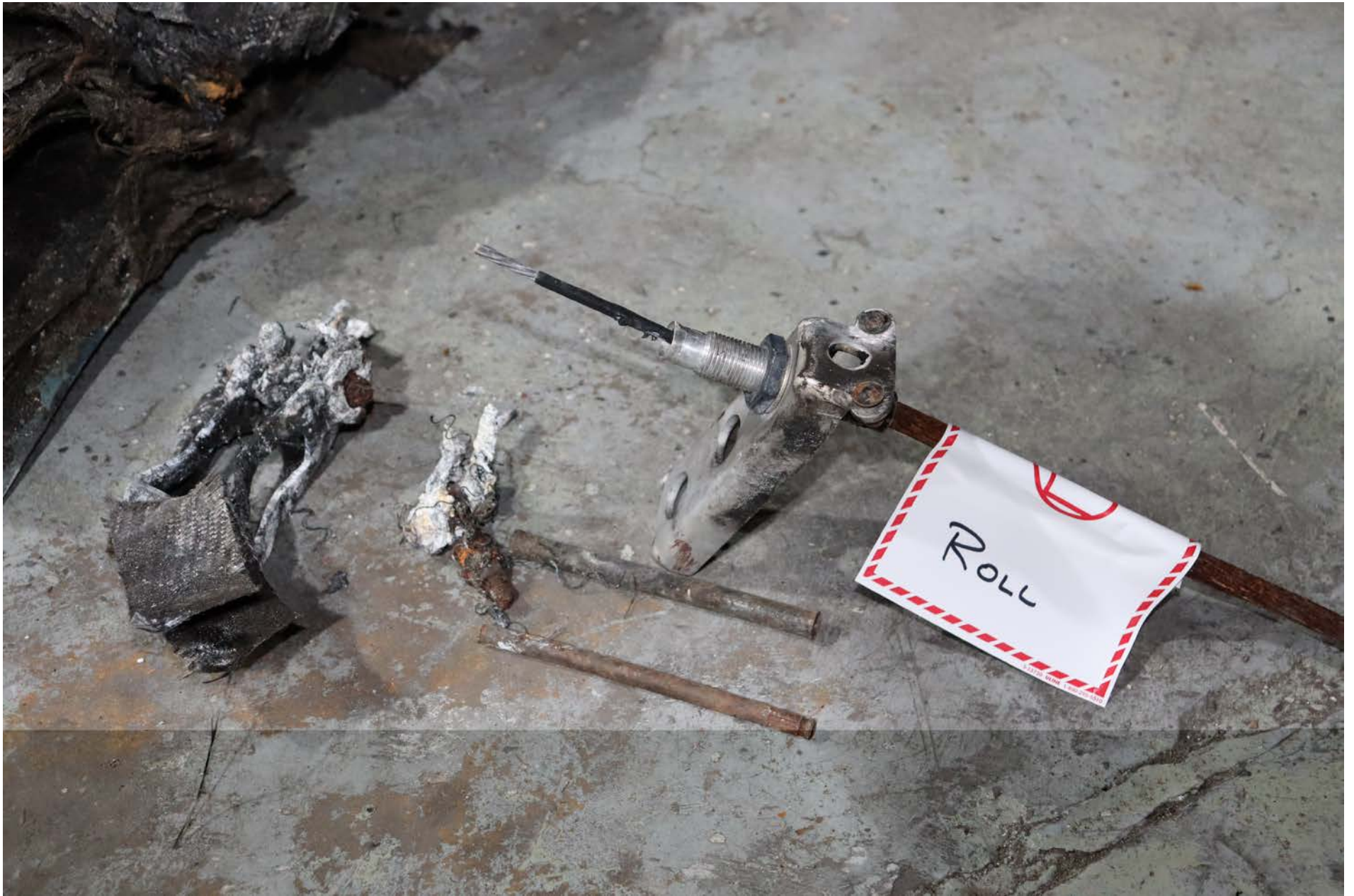
Photo 6 – View of Roll Cable, Sheath, Roll Control Clevis (AutoGyro USA)
