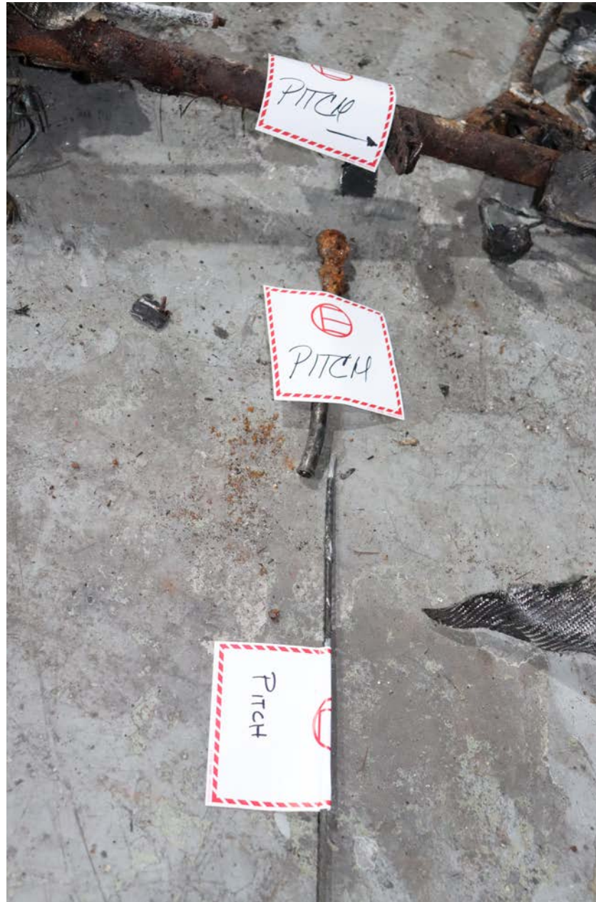
Photo 8 - View of Pitch Control Cable, Sheath, Rod-End Clevis, and Control Tube Pitch Horn (AutoGyro USA)
