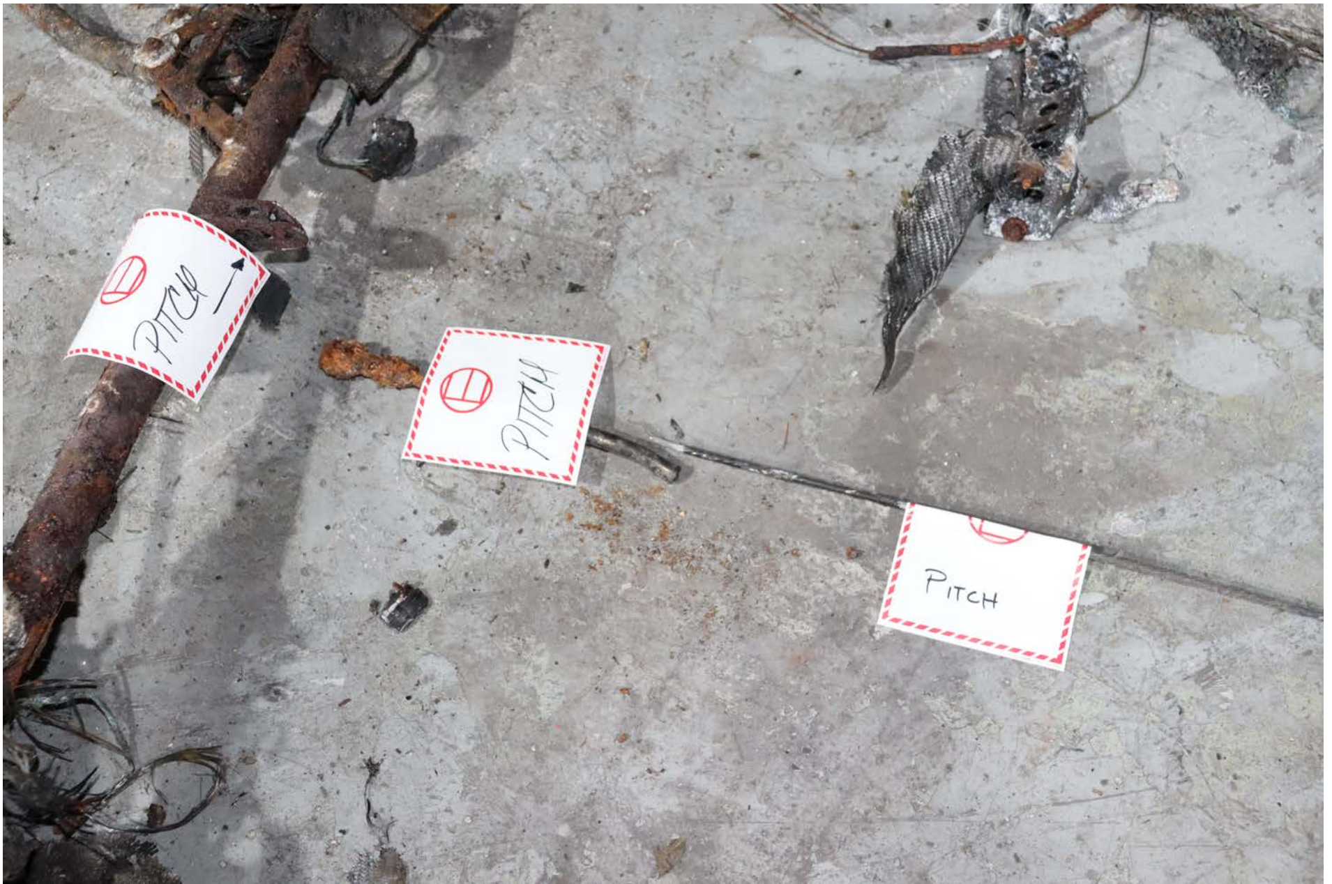
Photo 7 – View of Pitch Control Cable, Sheath, Rod-End Clevis, and Control Tube Pitch Horn (AutoGyro USA)
