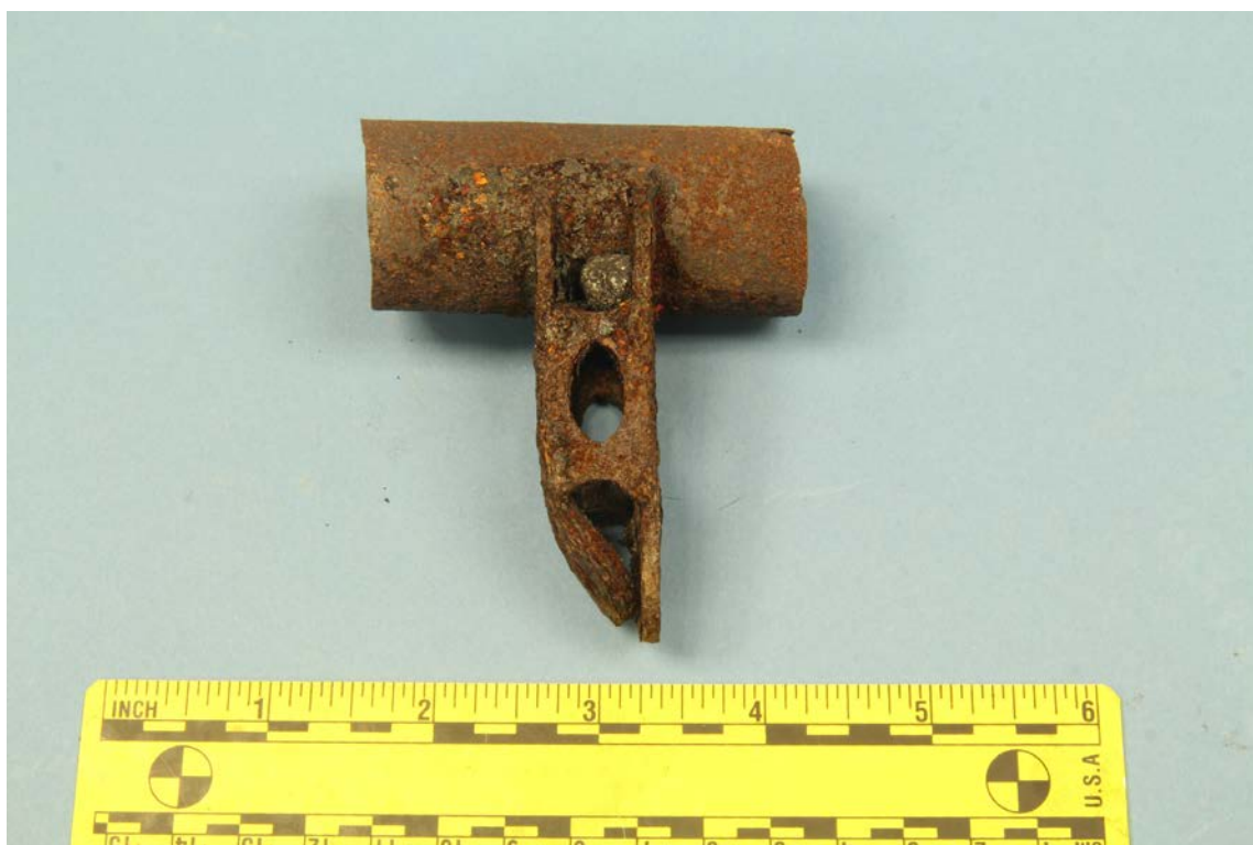
Figure 2: Pitch horn clevis with ear bent inwards.
