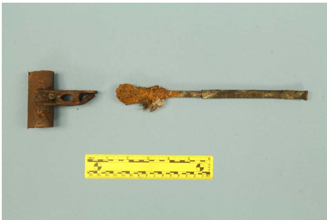
Figure 1: Pitch horn clevis and rod end as received.
