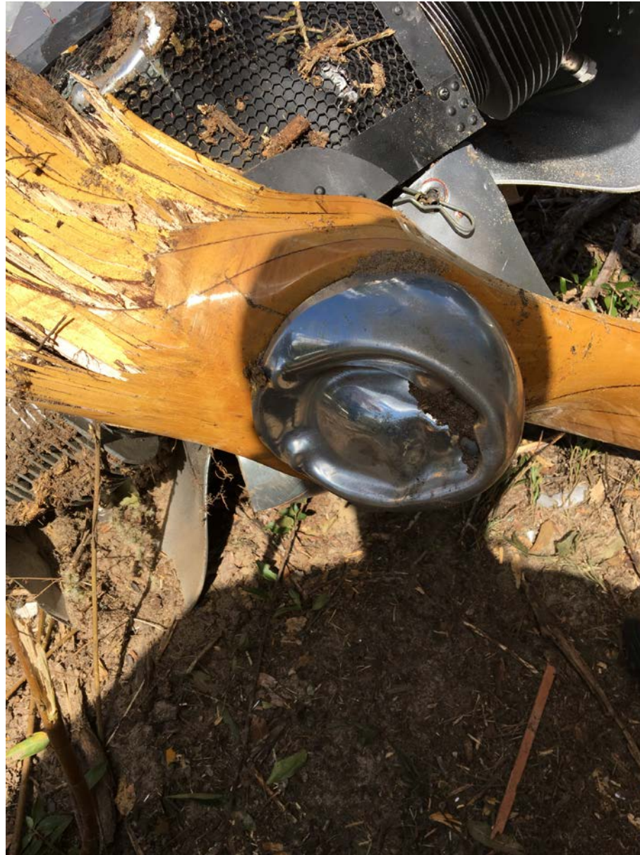
Photo 4 – View of propeller spinner and fractured propeller blades.
