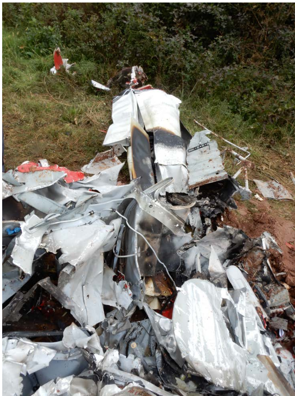
Photo 3 – View of cockpit and fuselage section
