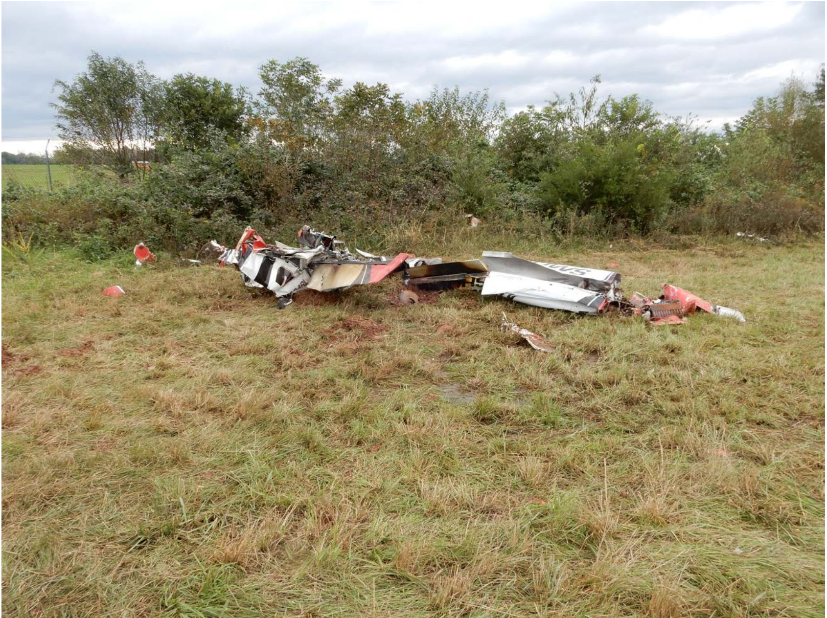
Photo 2 – View of right side of airplane wreckage showing parts of flight surfaces
