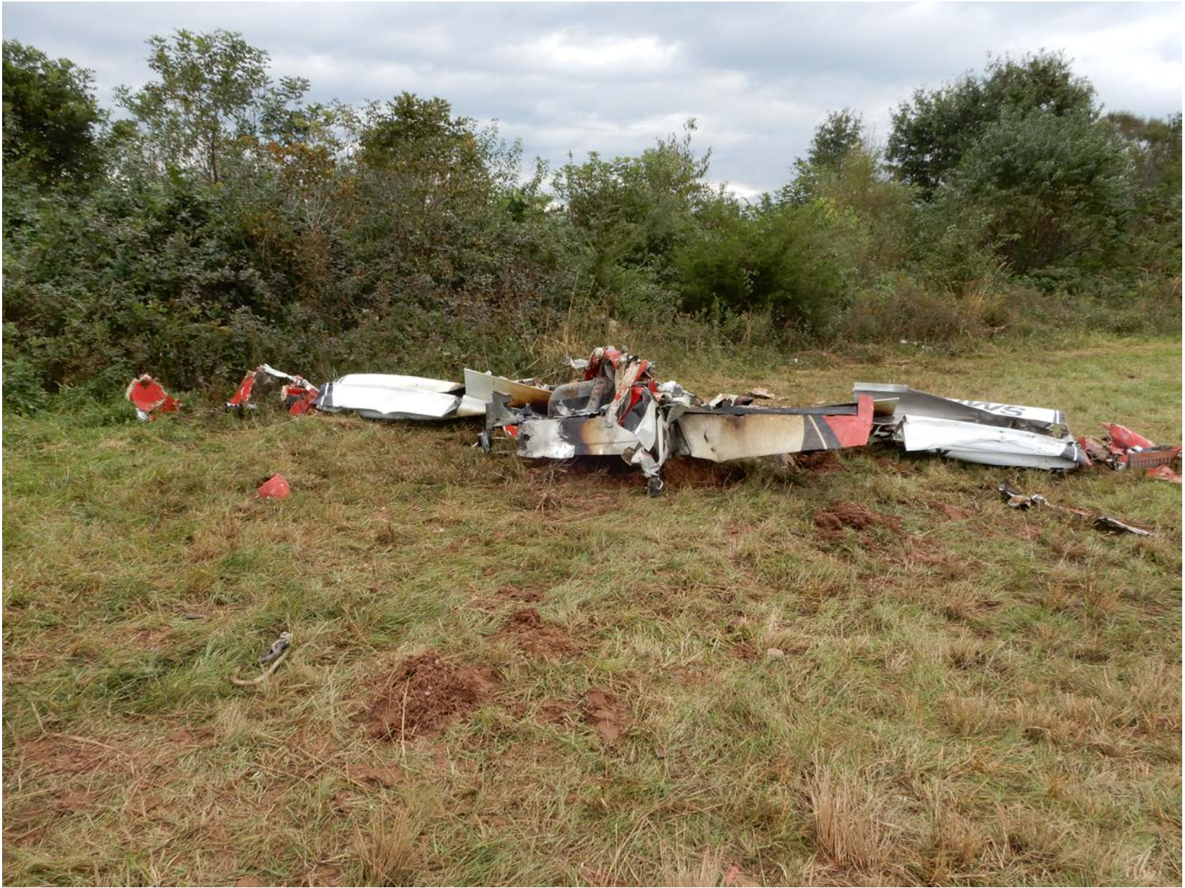
Photo 1 – View of aft of airplane wreckage showing damaged flight surfaces
