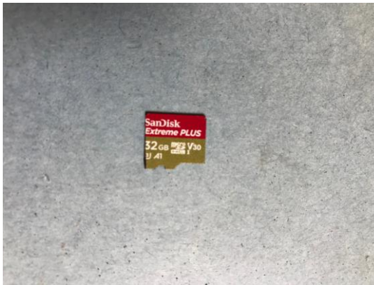
Figure 2. Photo of damaged microSD card. Notice the left side of the card is sheared off and missing.
