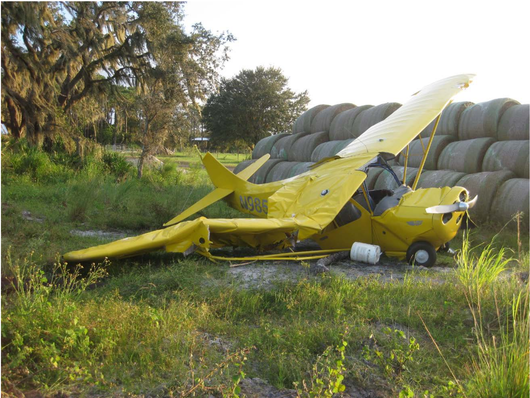
Photo 2 – Front right view of the airplane. (Photo courtesy of the FAA)
