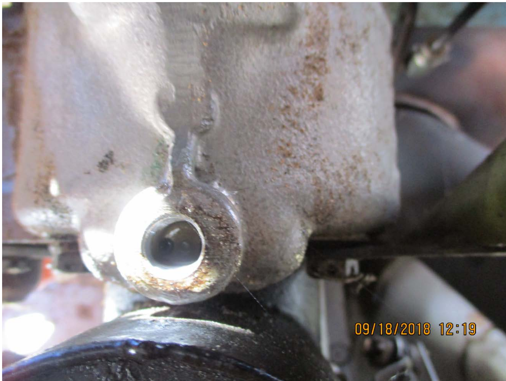
Photo 3 – Carburetor, plug missing
