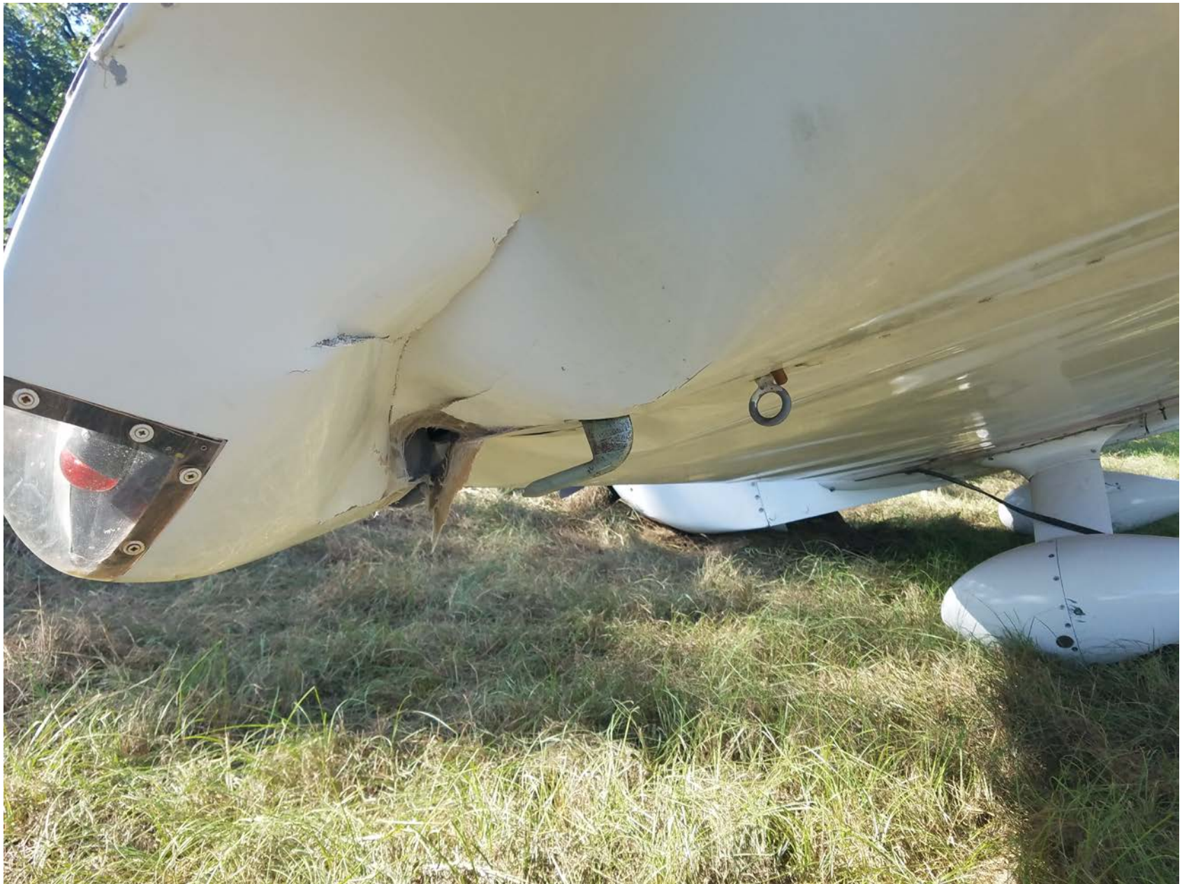
Photo 6 – Left-wing tip, wrinkled spar
