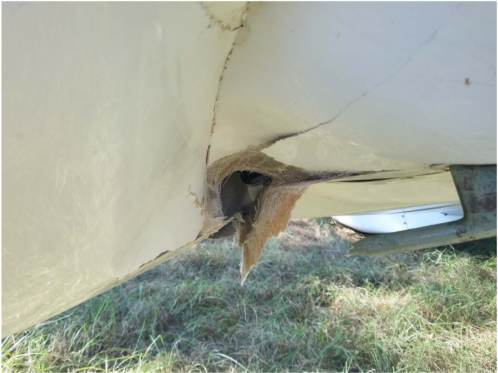
Photo 5 – left-wing tip, wrinkled spar
