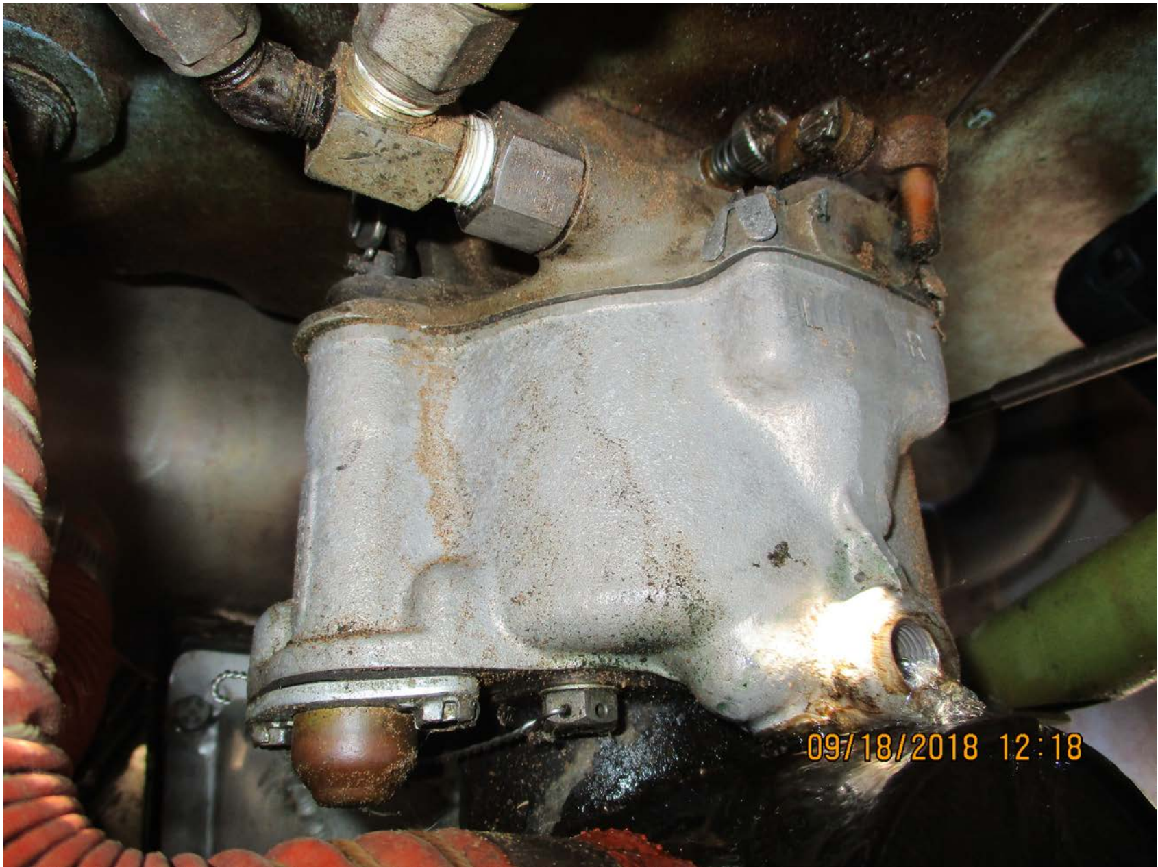
Photo 2 -Carburetor, fuel pouring out plug hole
