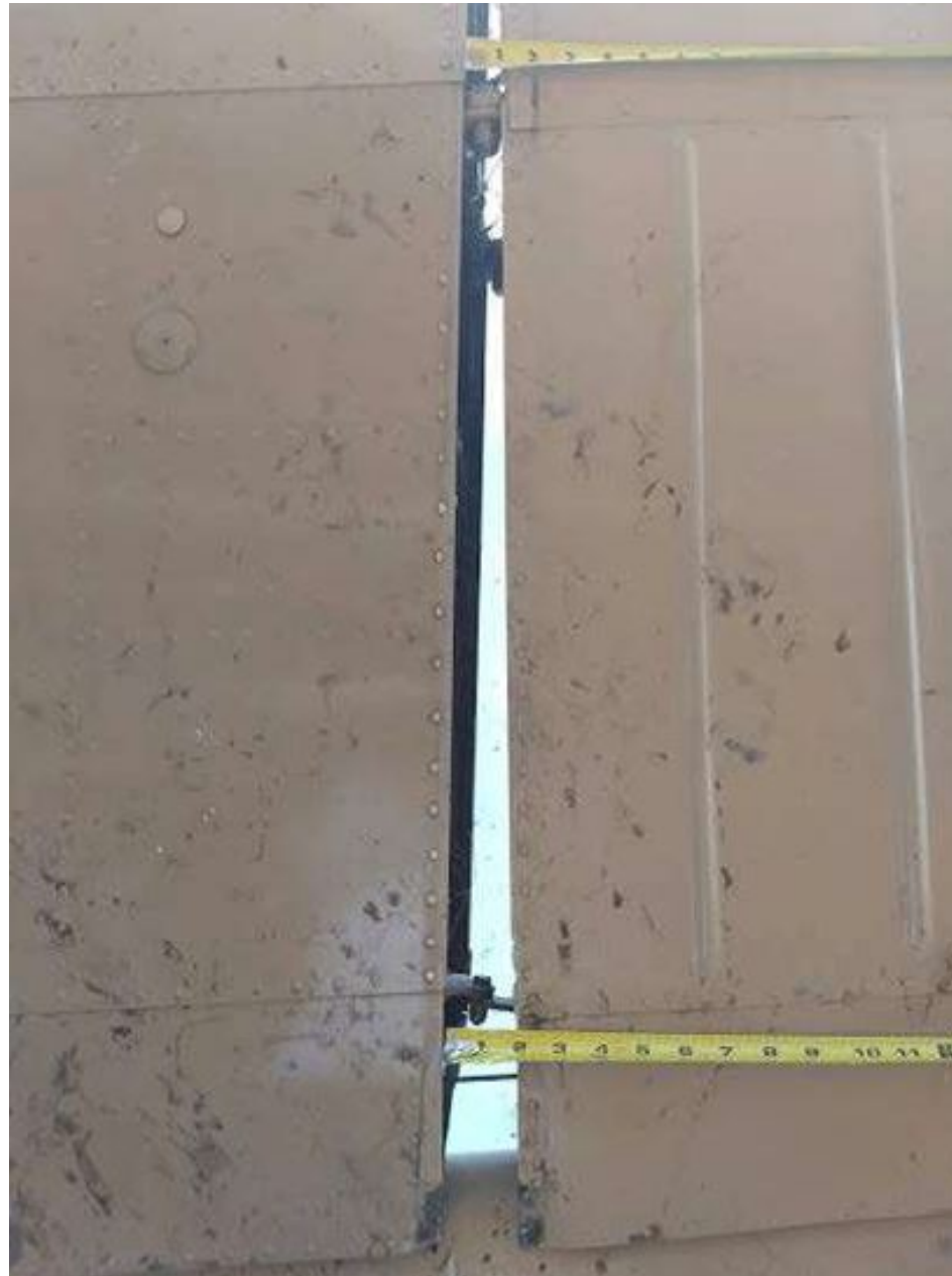
Photo 3 – Right Aileron Damage (Photo Courtesy of Bill Siegel, Mechanic)
