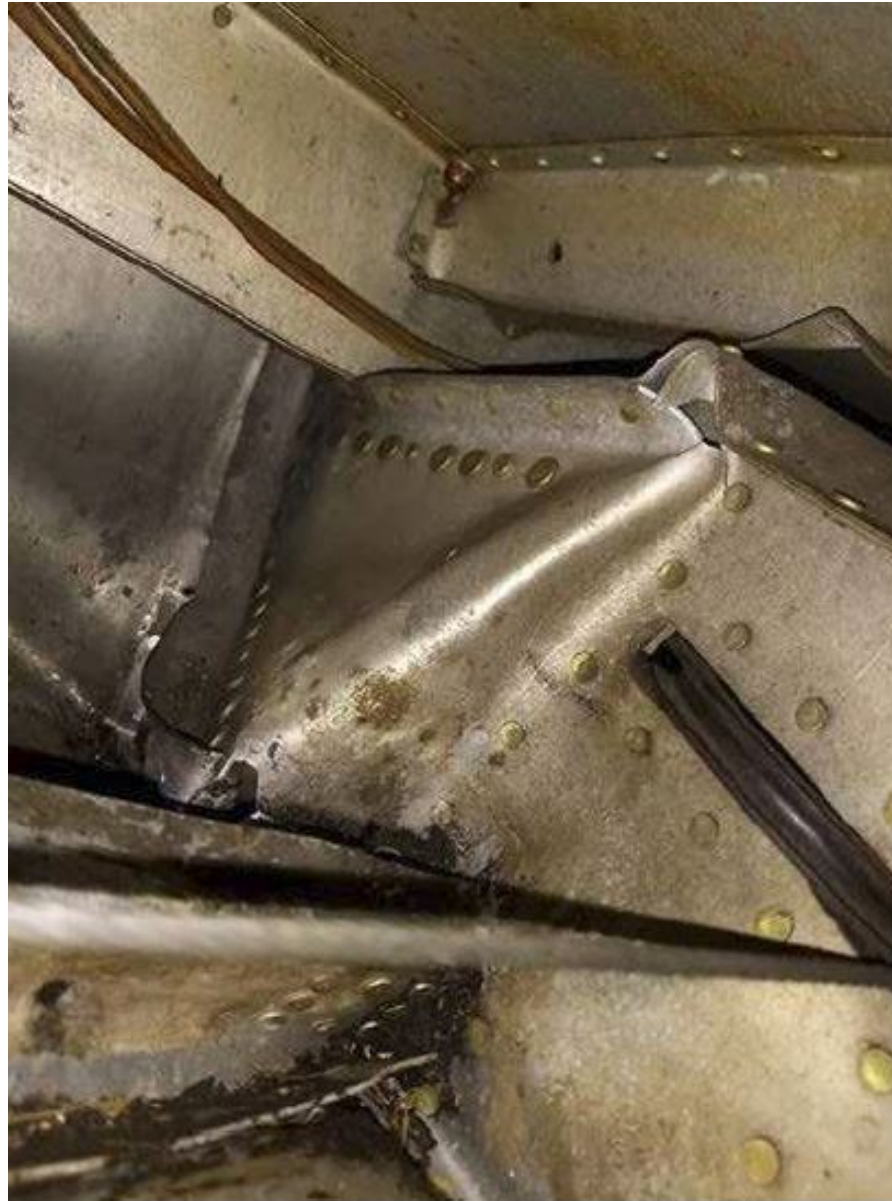
Photo 2 - Substantially Damaged Wing Spar Carry Through (Photo Courtesy of Bill Siegel, Mechanic)
