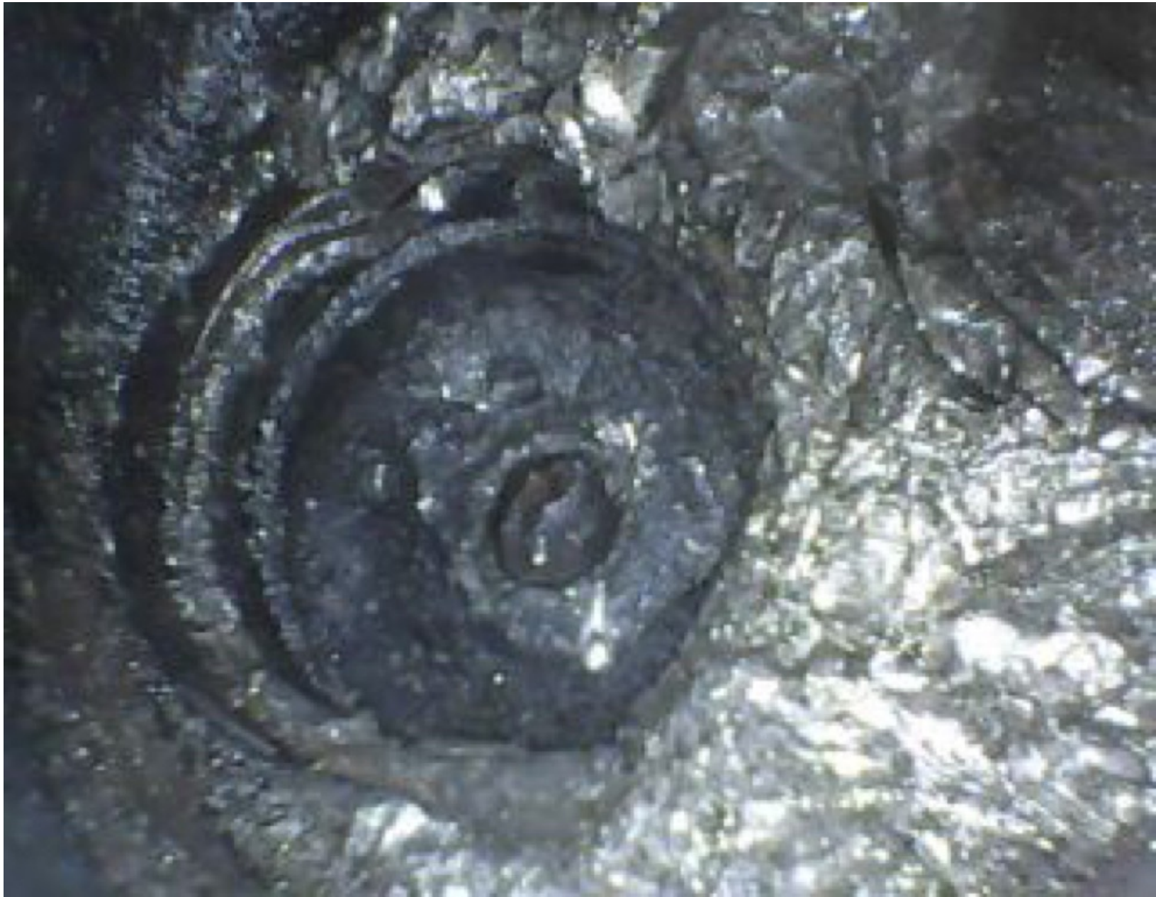
Photo 2 - #4-cylinder, fractured exhaust valve
