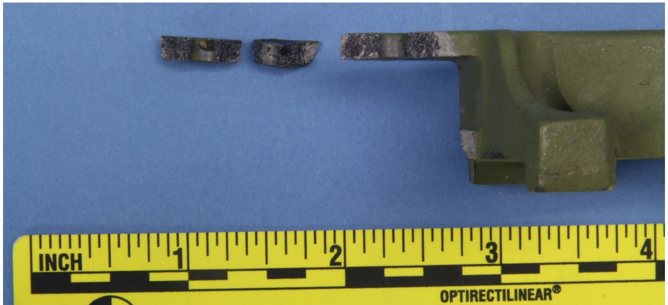
Figure 7 – View of the fractured clevis fracture surfaces, positioned to face the reader.
