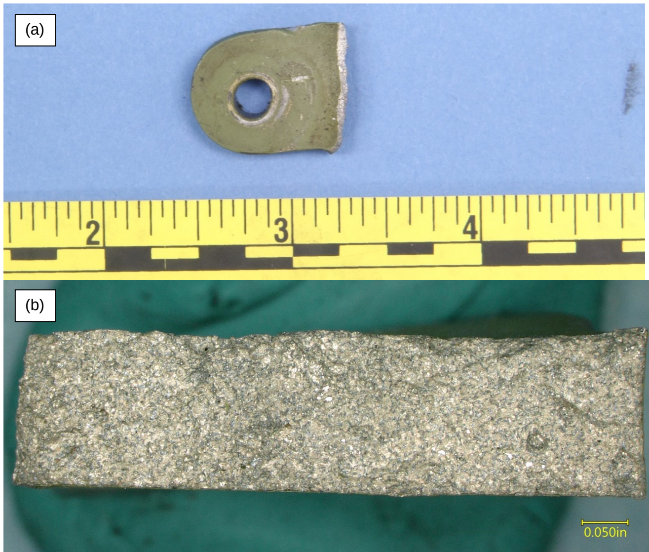
Figure 9 – View of the whole fractured clevis from (a) the side and (b) the fracture surface.
