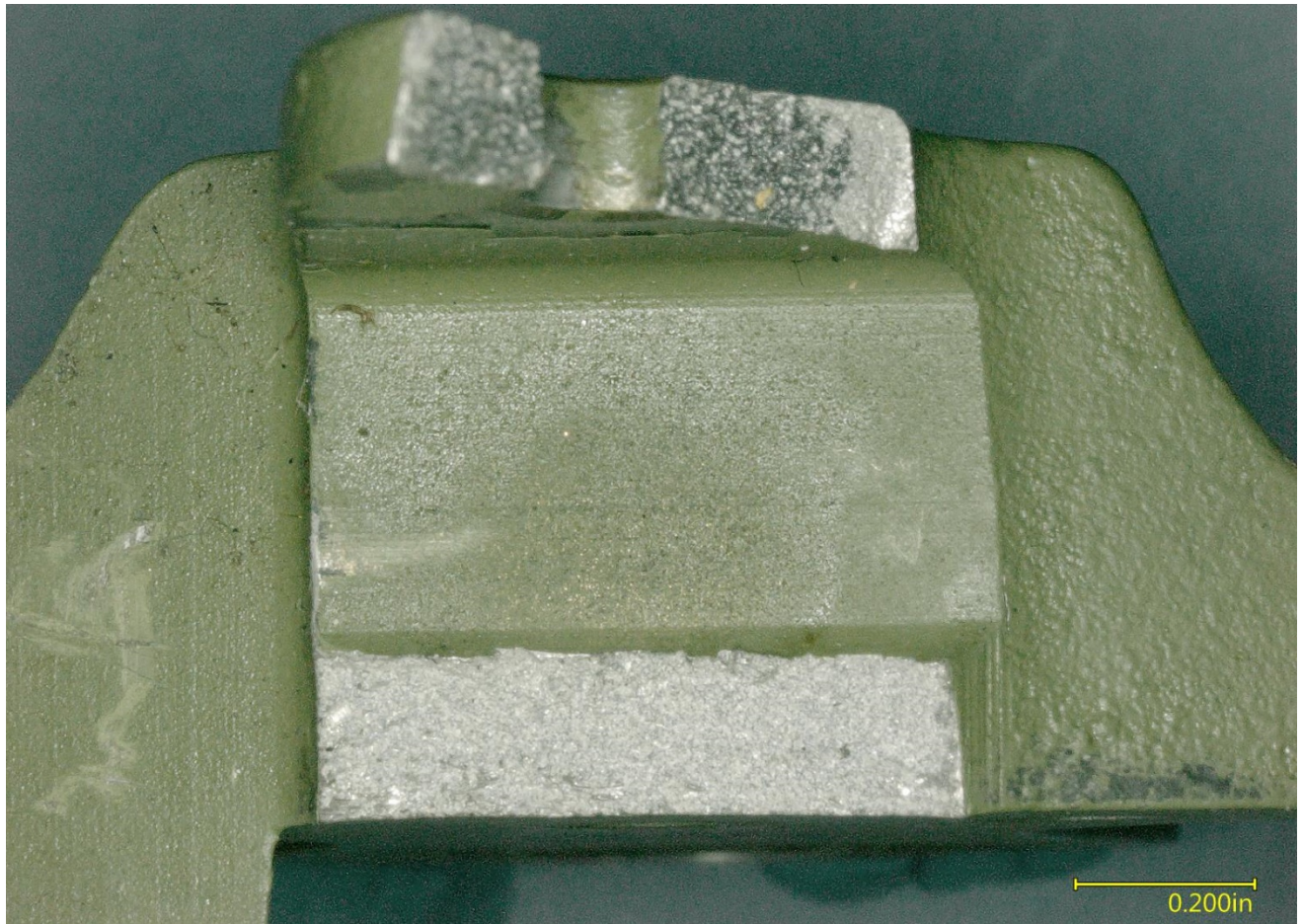
Figure 8 – The left pilot pedal arm from the forward side, tilted to show the clevis fracture surfaces.
