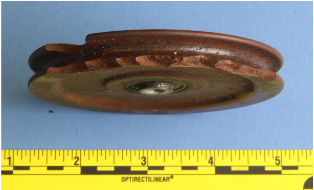
Figure 30 – View of the fracture surfaces of the pulley, as received.
