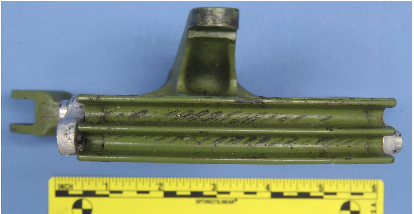
Figure 28 – View of the cable track of the bellcrank, showing impressions.
