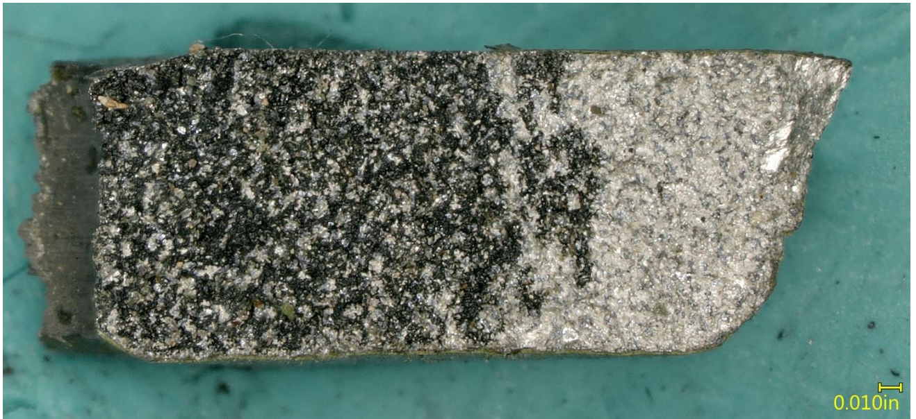
Figure 12 – Flat view of the fracture surface of the clevis fragment in Figure 11, showing dark and light regions.
