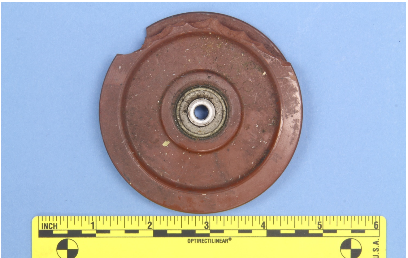
Figure 29 – The control pulley, as received.
