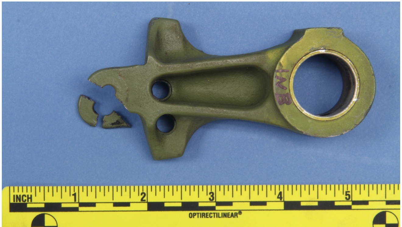
Figure 5 – The fractured pieces of the left pilot pedal arm from the inboard side.
