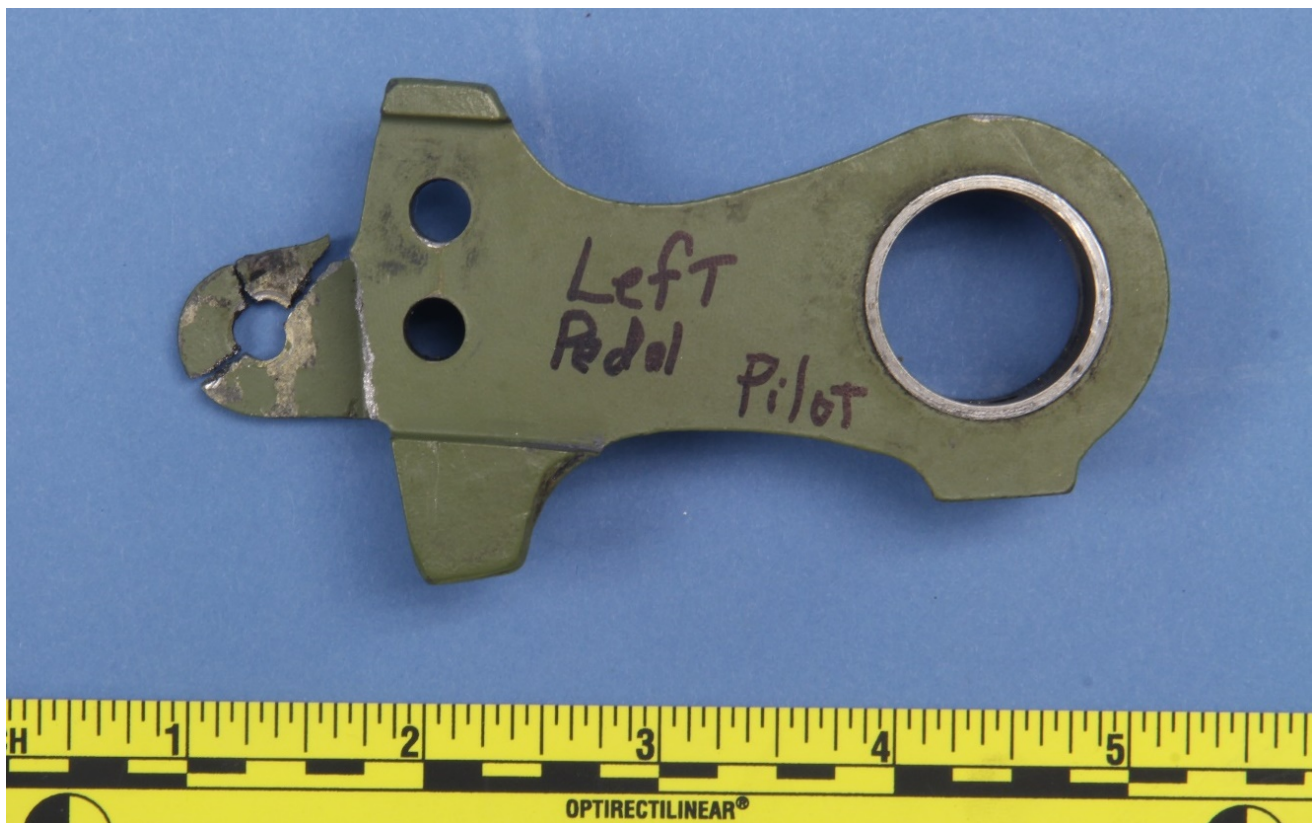
Figure 4 – The left pilot pedal arm from the outboard side, with the pieces of the fractured clevis positioned in their placement at fracture.
