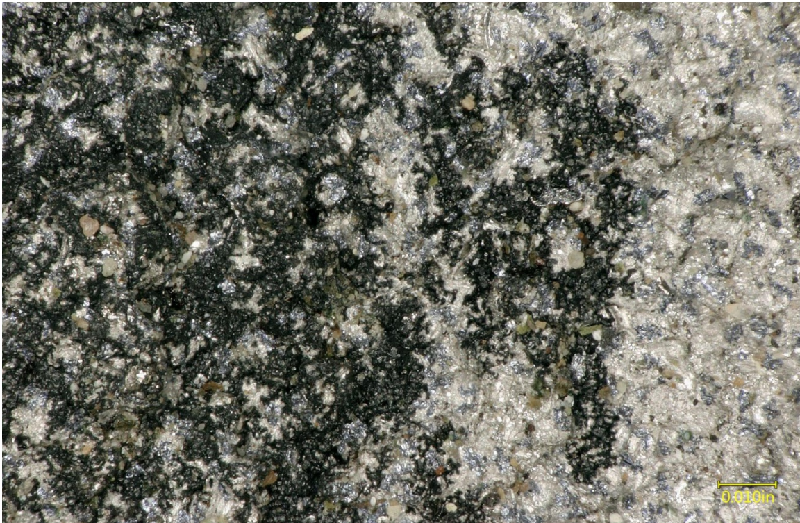
Figure 13 – Closer view of the fragment fracture surface, showing a dark surface material.
