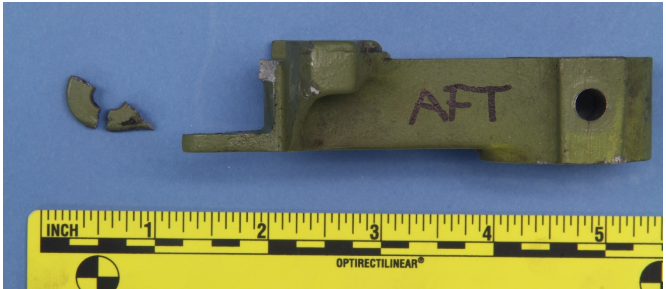
Figure 6 – The fractured pieces of the left pilot pedal arm from the aft side.
