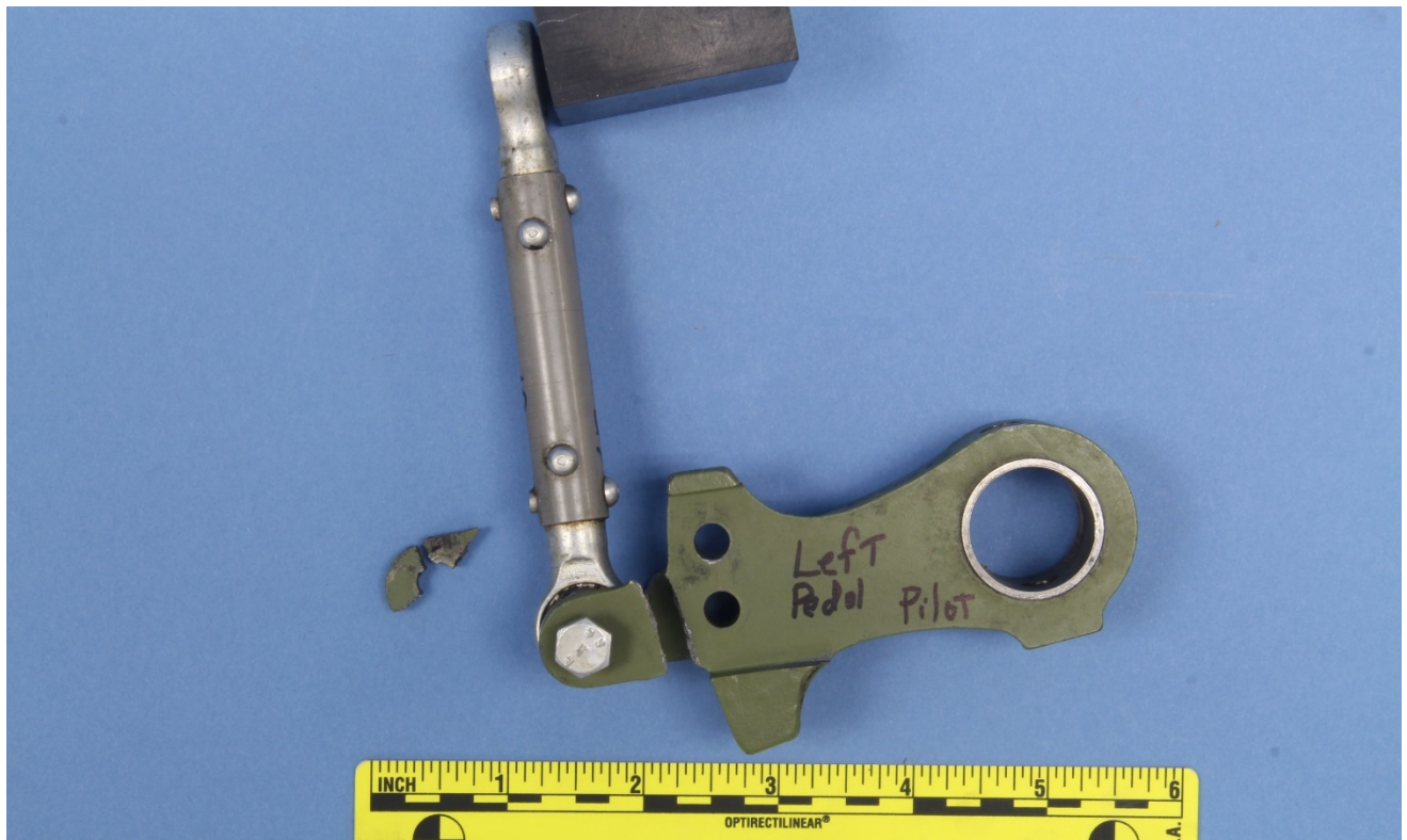
Figure 2 – The pilot left pedal from the outboard side, repositioned with the push rod tube to show placement of the fractured clevis attached to the rod bolt.
