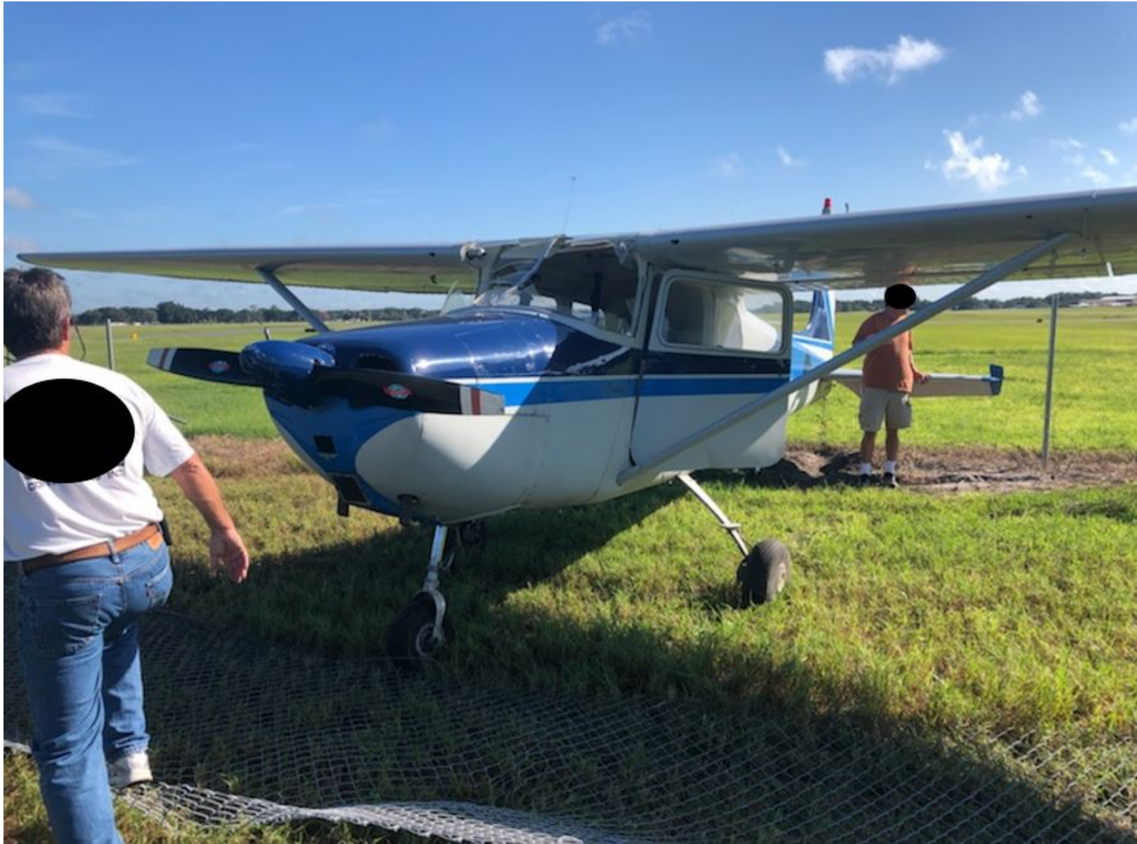
Photo 3 –Photograph of airplane, windshield, and fence damage. (Courtesy of FAA)
