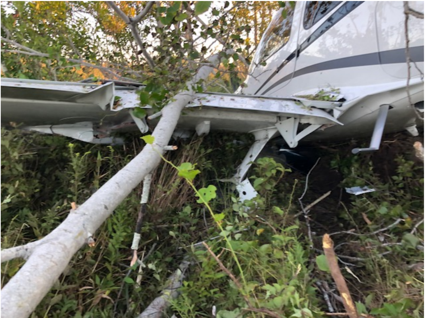
Photo 2 – View of Damage to Left Wing (FAA)
