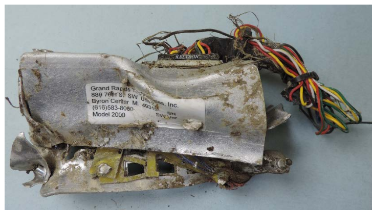
Figure 2. Grand Rapids Technology EIS 2000 as received.
