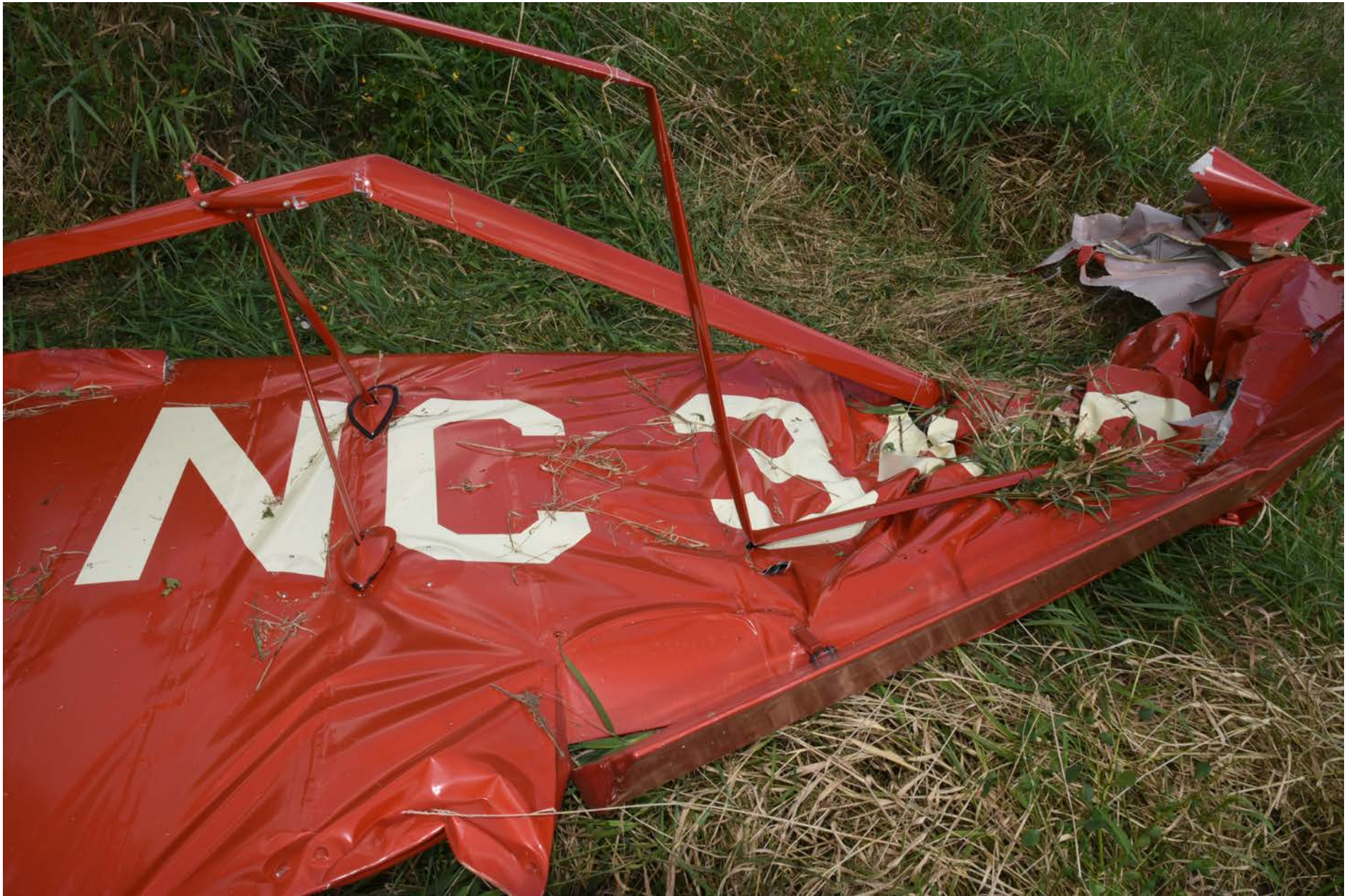
Photo 2 – View of left wing showing crush damage (Courtesy of FAA)
