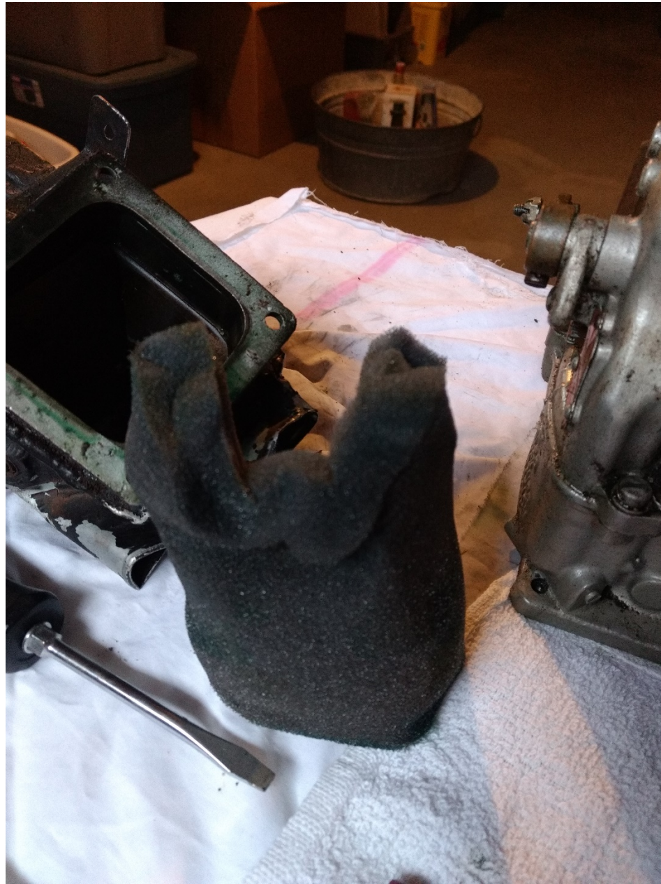
Photo 4 – View of Filter Removed from Carburetor (Courtesy of FAA)
