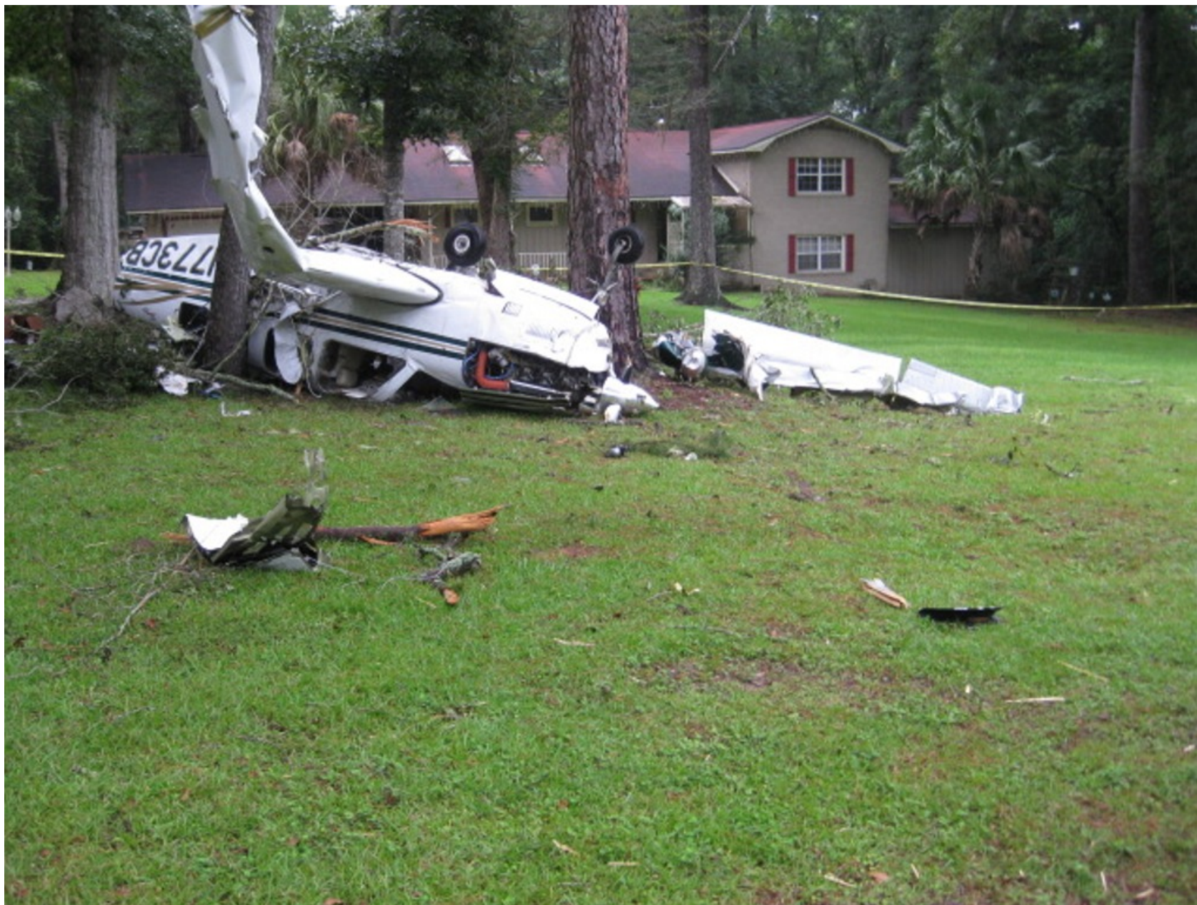
Photo 2 - FAA Digital Photograph. Left Forward Quartering View of the Inverted Wreckage at the Accident Site.
