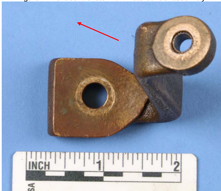
Figure 3: Control lever exhibiting plastic deformation. Red arrow shows direction of deformation.
