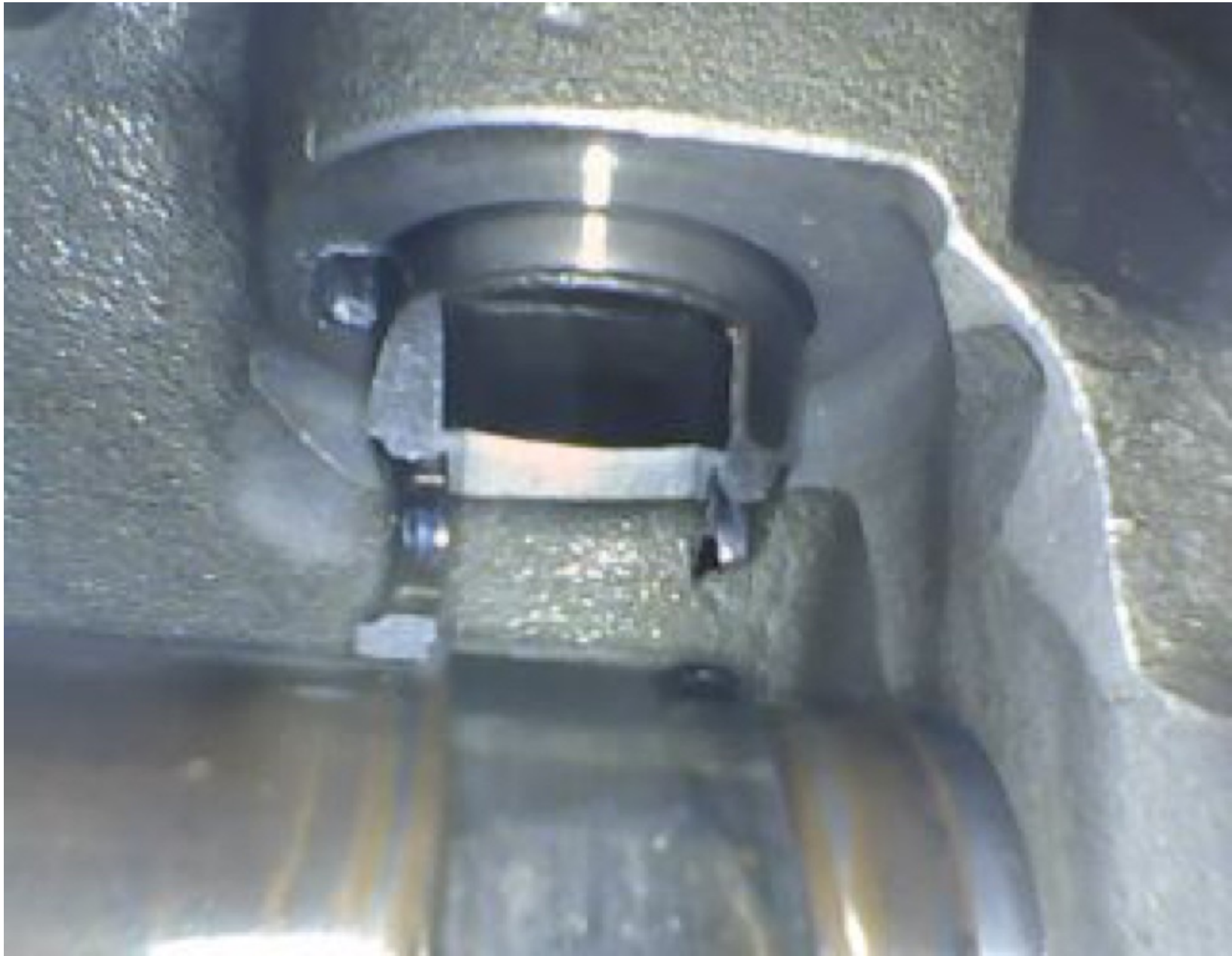
Photo 3 – Fractured roller tappet
