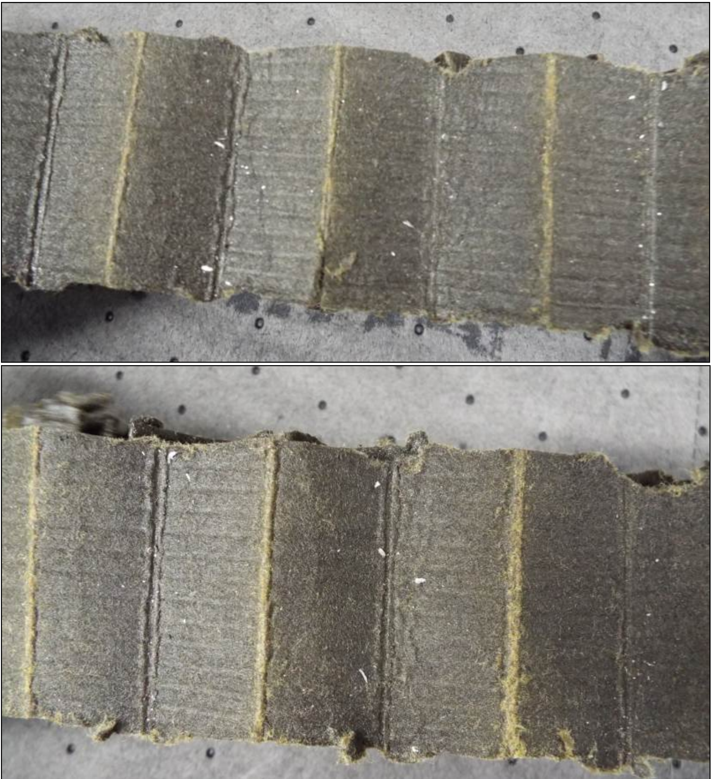
Figure 27. Typical regions showing the amount of chips found in the oil filter upon examination.
