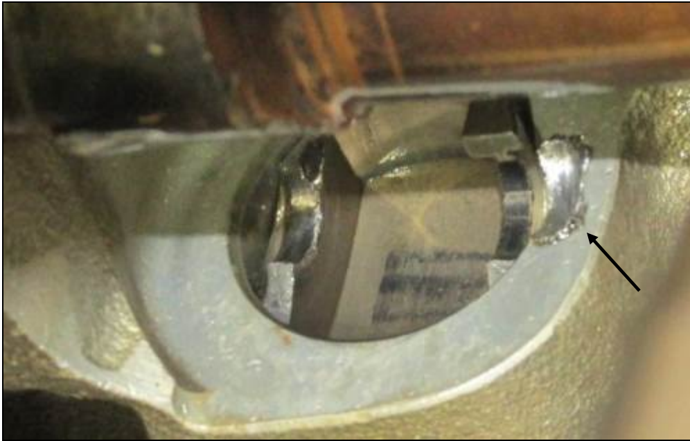
Figure 1. Witness mark in crankcase likely from the roller shaft based on the diameter and position. (Photo from SIR image file)
