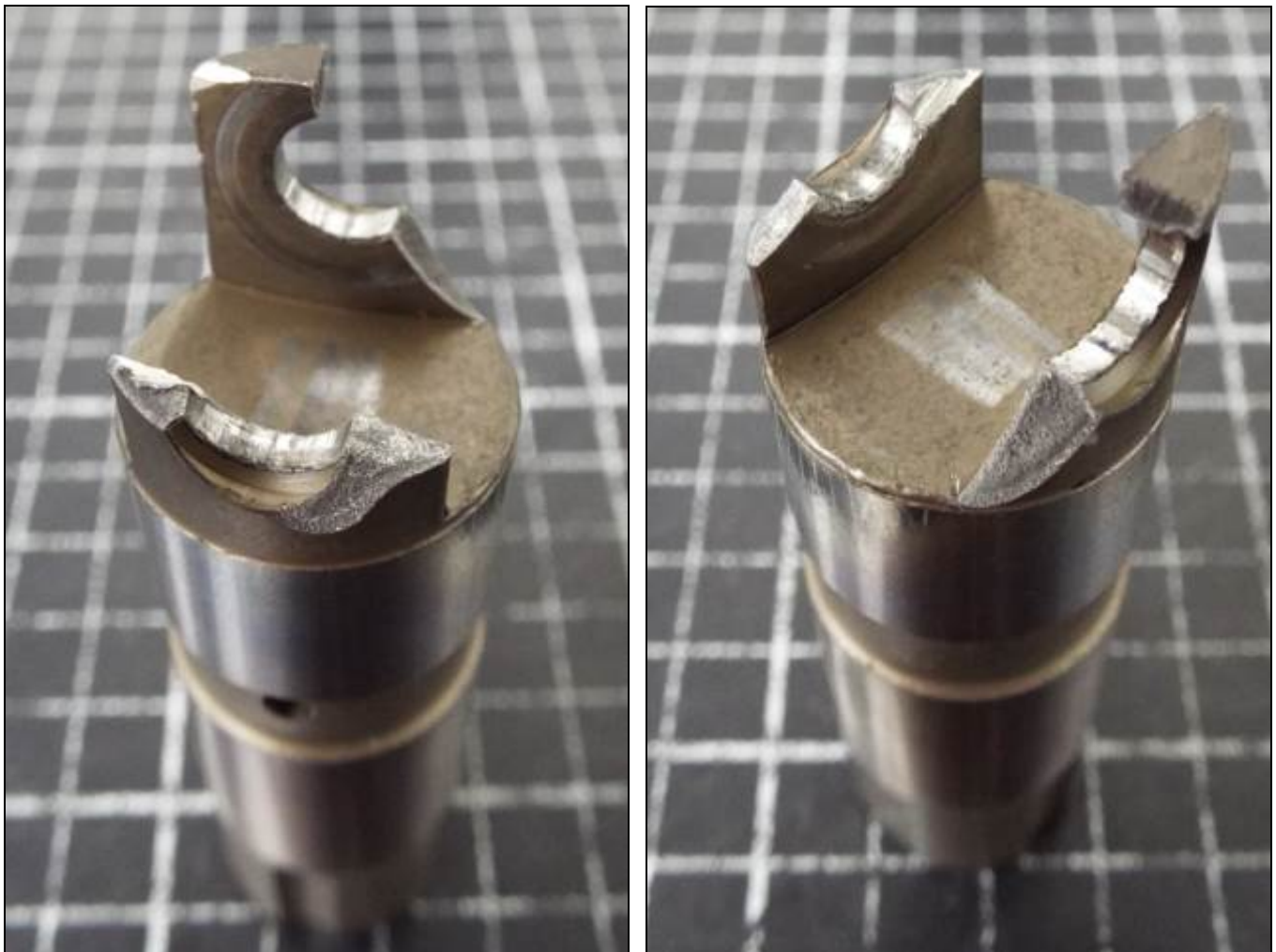
Figure 13. Macro photos of the fractured #4 exhaust roller tappet assembly.
