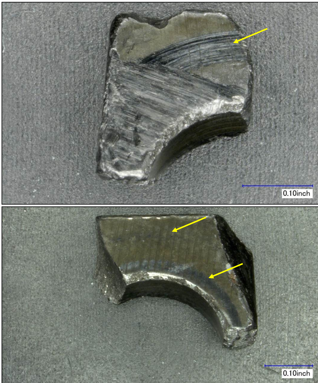
Figure 15. Witness marks from the roller and needle bearings.
