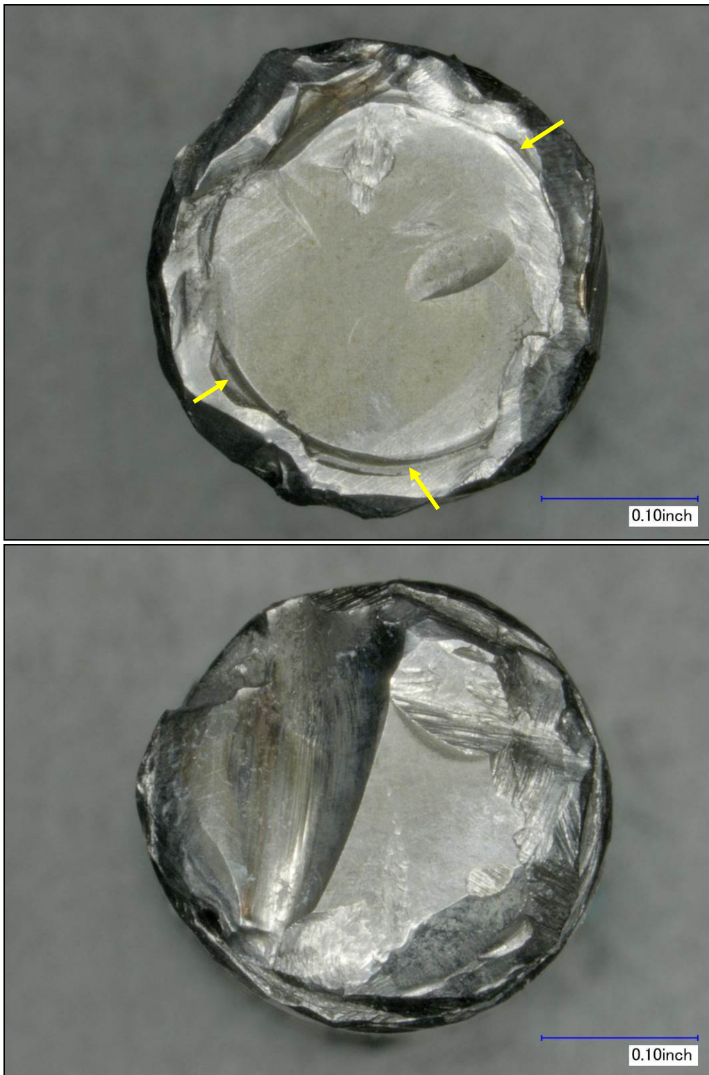
Figure 25. Both ends of the shaft are shown. In the top image, yellow arrows indicate the indent from the staking operation. In the bottom image, the opposite end of the shaft is badly damaged.
