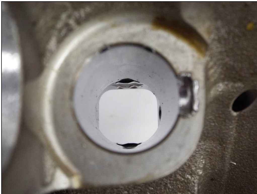
Figure 4. Crankcase tappet bore of #4 exhaust roller tappet, viewed from inside of case, with no abnormal wear.
