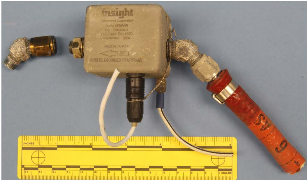
Figure 1 Image of the as-received portion of a fuel transducer and a portion of a fuel line with AN fitting.
